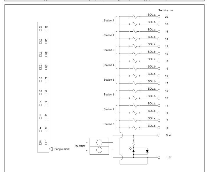
Note 1) This circuits are for the specifications with up to 8 stations of 2 position double, 3 position and 4 position dual 3 port valves. These should be wired in order 20→18→16→14 without skipping or leaving any connectors remaining.
