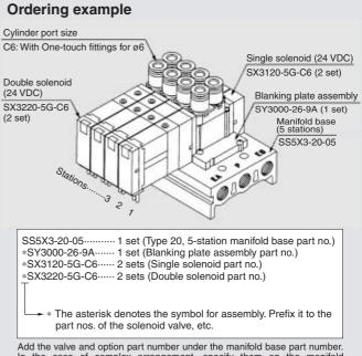
Add the valve and option part number under the manifold base part number. In the case of complex arrangement, specify them on the manifold specification sheet.
