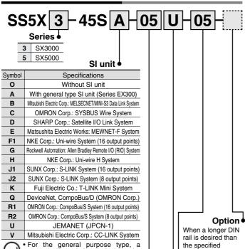
For the general purpose type, a transmission unit is required on the CPU side.
