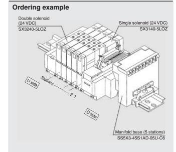
SS5X3-45S1AD-05U-C6··· 1 set (45S1 with serial 5-station manifold base no.) \*SX3140-5LOZ.....2 sets (Single solenoid part no.) \*SX3240-5LOZ-----3 sets (Double solenoid part no.)
