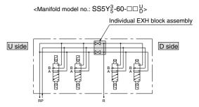
[When a separate exhaust passage is needed on only a middle valve.] Specify arrangement of individual EXH block assembly and EXH block disk on the manifold specification sheet.
