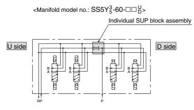
[When a different supply pressure is required for only a middle valve.] Specify arrangement of individual SUP block assembly and SUP block disk on the manifold specification sheet.
