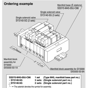
Prefix it to the part nos. of the solenoid valve, etc.
