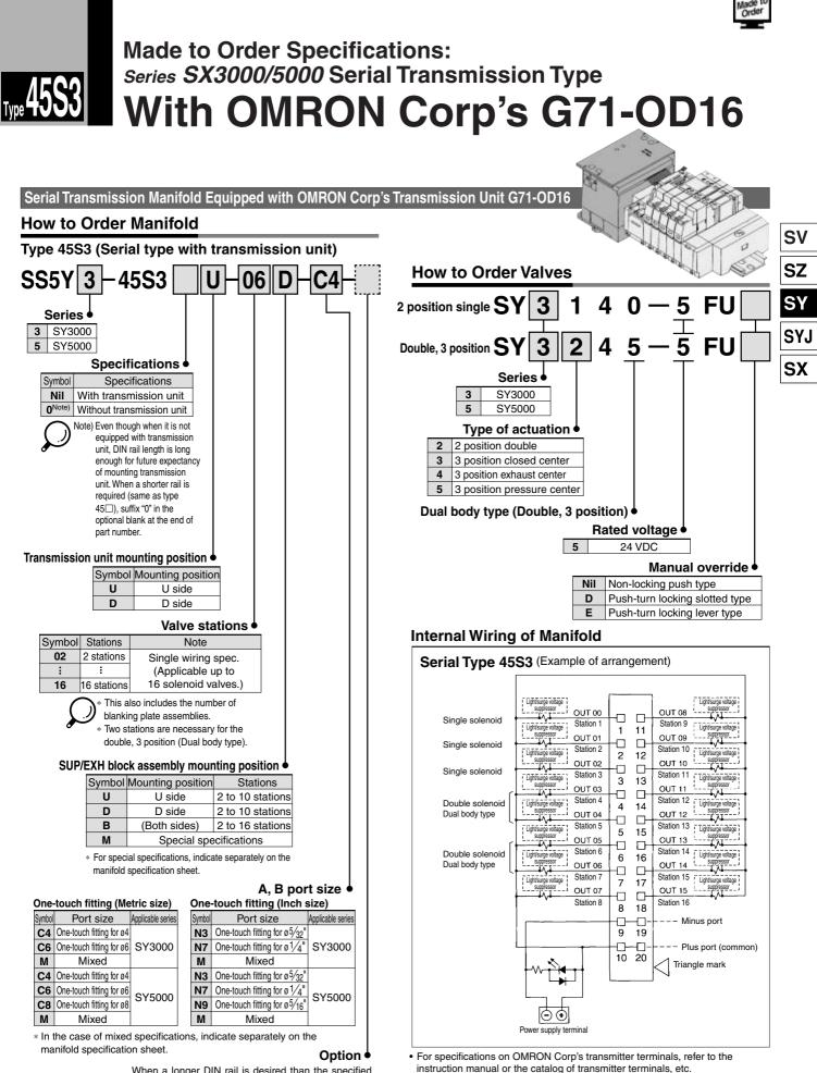
When a longer DIN rail is desired than the specified stations, specify the station number to be required. (20 stations at maximum)
