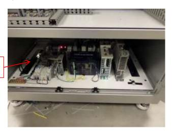
The 120 VAC electrical plug can be routed through this slot.
