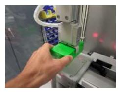
7. If a Stepper or Servo Controller error occurs (example, after a jam), the power needs to be cycled off then on to clear. When three unsuccessful resets fail to home the machine, all four amber lights in the window will flash indicating the power needs to be cycled to clear. When cycling the power, leave the power off at least 10 seconds prior to restoring power.
