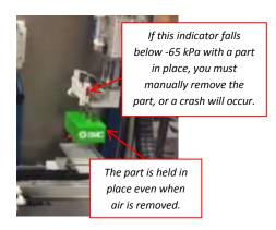
9. Four of the 3 position SY Valves have an open center (see illustration below). During a catastrophic loss of the main air supplied to the unit, these valves could stop in a floated position where the pilot cannot actuate in either direction. The manifold will sound with a solid hiss. In this situation, you may need to remove the faulting valve from the manifold, and manually move the spool one way or the other.
