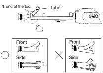
2. After inserting, grasp the handle tightly and insert the end of the tubing to the stroke end.
