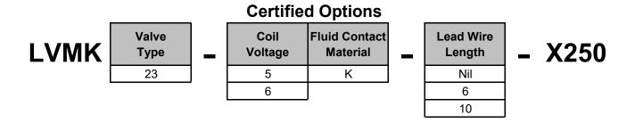
Note: X250 signifies cURus certification on the standard valve. Must order with X250 to have the UL Mark.
