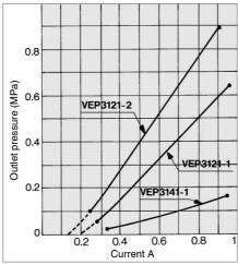
Pressure Characteristics JIS B 8372 (In accordance with air regulator)
