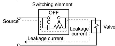
Ensure that voltage leakage across the coil as follows :
