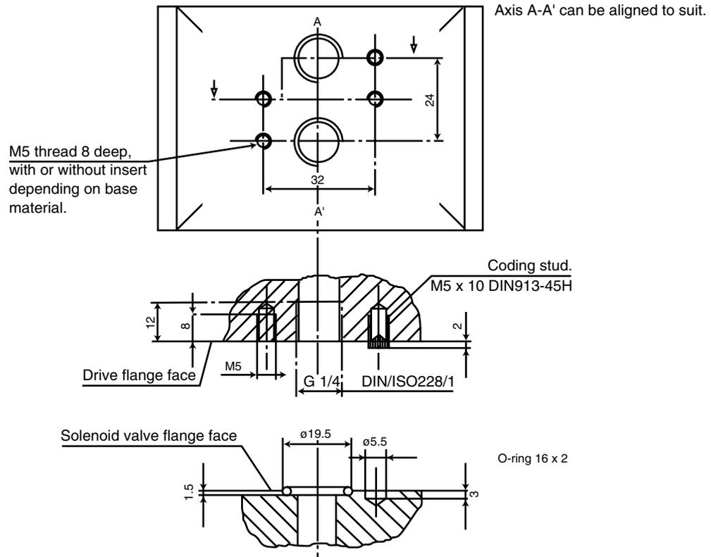
The solenoid valve can be attached with 2 mounting bolts.
