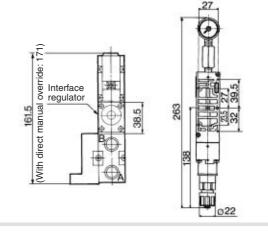
Interface regulator/B port regulation: ARBF3050-00-B-1 (Plug-in type) ARBF3050-00-B-2 (Non plug-in type)
