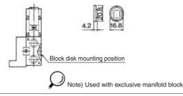
Throttle valve spacer: VVFS3000-20A-1 (Plug-in type) VVFS3000-20A-2 (Non plug-in type)
