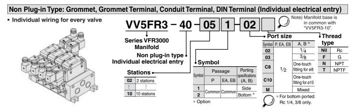
Note) Manifold base is in common with Series VFS3000.
