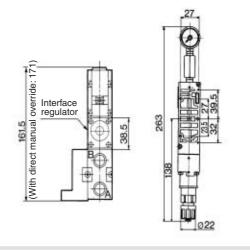
Interface regulator/A port regulation: ARBF3050-00-A-1 (Plug-in type) ARBF3050-00-A-2 (Non plug-in type)
