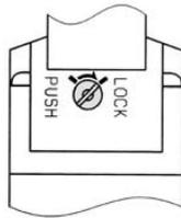
Push the manual override button with a small flat head screwdriver until it stops. Turn it in the clockwise direction at 90° to lock the manual. Turn it counterclockwise to release it.
