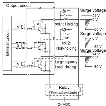
Figure 1. Surge intrusion circuit example (NPN outlet example)
