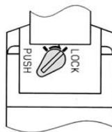
After pushing down, turn in the direction of the arrow. If it is not turned, it can be operated the same way as the non-locking type.
