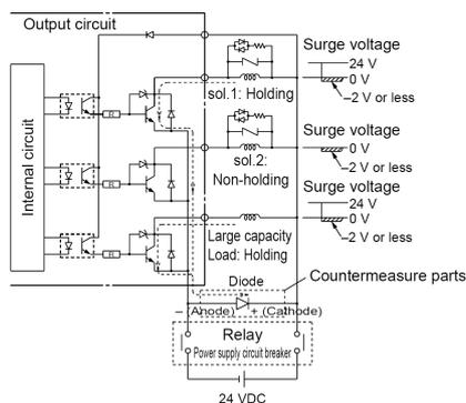
Figure 2. Surge intrusion circuit example (NPN outlet example)
