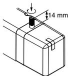
Push down the manual override button with a small flat head screwdriver or with your finger until it stops, and turn it clockwise 90° to lock it. Turn it counterclockwise to release it.
