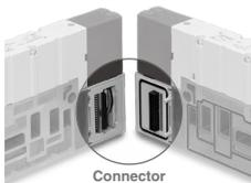
(Refer to the connector wiring diagram.) Printed circuit board patterns between connectors are shifted at every station. This allows for viable connections to take place without necessarily specifying whether the manifold station is double, single, or mixed wiring.
