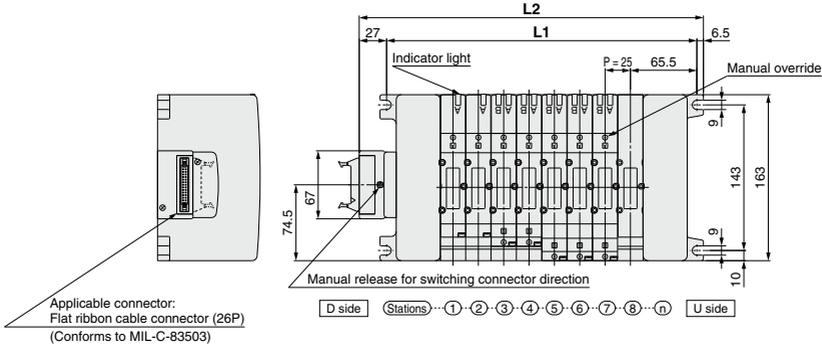
Flat ribbon cable connector assembly (26P)
