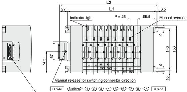
Applicable connector: D-sub connector (25P)
