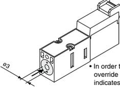
• In order to turn it ON, push down the manual override button in the direction the arrow (→) indicates until it stops (approx. 0.5 mm), and release it to turn it OFF.
