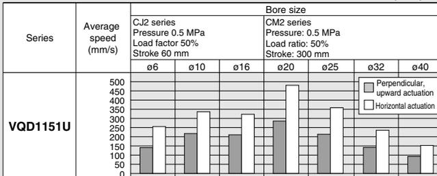
\* It is when the cylinder is extending that is meter-out controlled by speed controller which is directly connected with cylinder, and its needle valve with being fully open.
