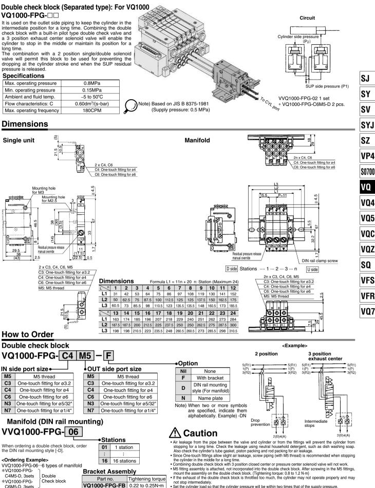
not stop intermediately. • Set the cylinder load so that the cylinder pressure will be within two times that of the supply pressure
