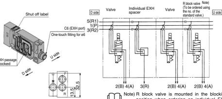
Note) R block valve is mounted in the blocking position when ordering an individual EXH spacer incorporated with a manifold. When separately ordering an individual EXH
