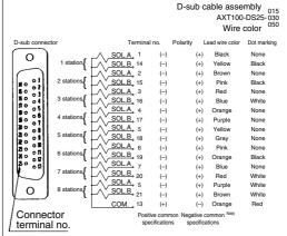
As the standard electrical wiring specifications, double wiring (connected to SOL. A and SOL. B) is adopted for the internal wiring of each station for 8 stations or less, regardless of valve and option types. Mixed single and double wiring is available as an option. For details, refer to page 2-4-69.
