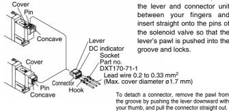
To attach a connector, hold the lever and connector unit between your fingers and insert straight onto the pins of the solenoid valve so that the lever's pawl is pushed into the groove and locks.
