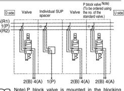
Note) P block valve is mounted in the blocking position when ordering an individual SUP spacer incorporated with a manifold. When separately ordering an individual SUP spacer, separately order a P block valve.
