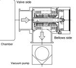
The valve may not be mounted depending on the piping material type (clamp, etc.). Be sure to check the piping material before use.
