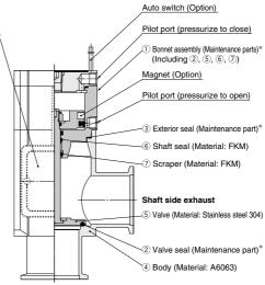
Valve side exhaust \* Refer to the back of page 465 for "Maintenance Parts".
