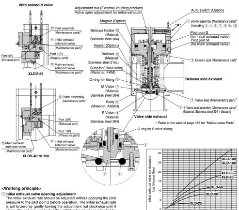
stops. (Do not use any tools.) The initial exhaust rate is adjusted by turning the adjustment nut counterclockwise. 2 Opening of the initial exhaust valve (valve S) When the pilot pressure is applied to the pilot port S, the valve S is
