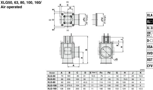
Note 1) Dimension E applies when heater option is included. (Lead wire length: approx. 1 m)
