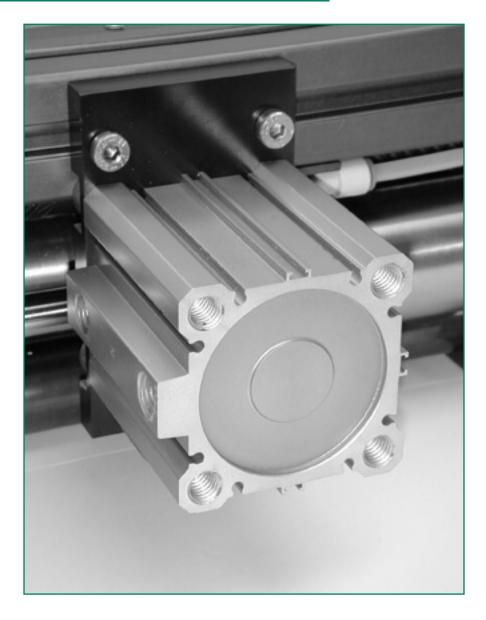
In applications that require the part be held even when pneumatic power is lost, the Power-Off Brake option provides an excellent solution. When pneumatic pressure is removed from the option a spring is allowed to rotate a collar that engages a collet brake system on the helix. Thus, the jaws are braked in position.
