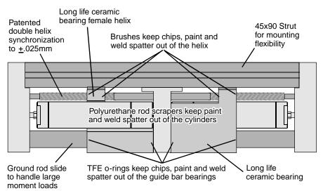
The synchronous XRAY utilizes U.S. patent numbers 4,591,199 and 5,657,973. The force and synchronizing double helix are independent systems. The double helix works only to center the part to .025mm ( $\pm$ 0.001inches). All of the gripping force is provided by two pistons that are driven pneumatically. The independence of the force and synchronization systems provides precision over the typical 10,000,000+ cycle life of the unit.
