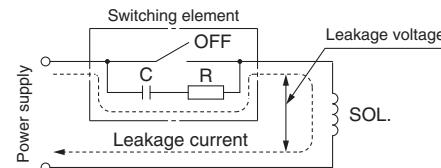
AC coil: 5 % or less of the rated voltage
