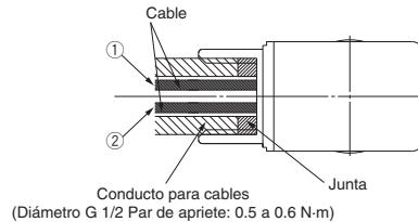
Wiring conduit (Bore size G1/2 Tightening torque 0.5 to 0.6 N·m)
