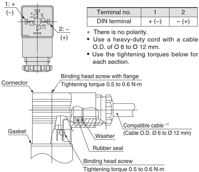
\*1 For cables with an O.D. of Ø 9 to Ø 12 mm, remove the internal parts of the rubber seal before using.
