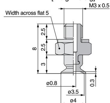
Pad diameter  $\phi 1.5$  to  $\phi 3.5$
