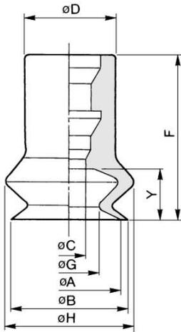
Pad diameter:  $\phi 10$  to  $\phi 50$
