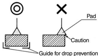
If multiple pads are used for transferring a flat object with a large surface area, properly allocate the pads to maintain balance. Also make sure that the pads are aligned properly to prevent them from becoming disengaged along the edges.
