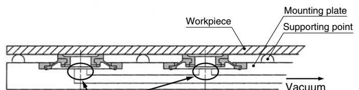
When a hole is made in the plate, the dimension shall be (\*) or less.
