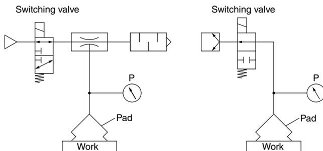
**Vacuum Pressure and Response Time after Supply Valve (Switching Valve) is Operated**
