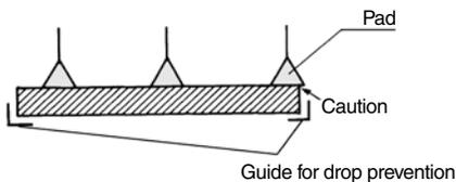
Provide an auxiliary device (example: a guide for preventing the workpieces from dropping) as necessary.
