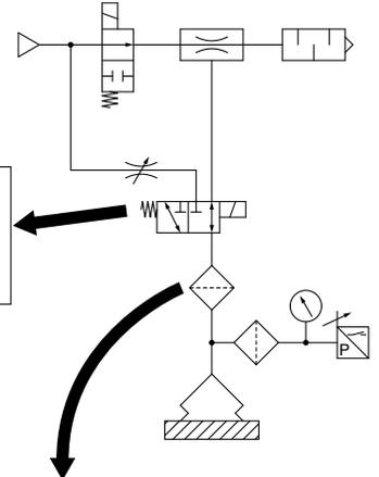
Use a suction filter (Series ZFA, ZFB, ZFC) to protect the switching valve and to prevent the ejector from becoming clogged. Also, a suction filter must be used in a dusty environment. If only the unit's filter is used, it will become clogged quickly.
