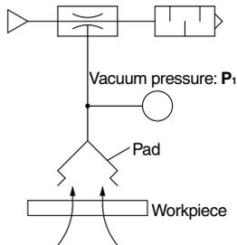
**Exercise:** Using a supply pressure of 0.45 MPa, when the ejector (ZH07□S) picks up a workpiece that leaks air, the vacuum gauge indicated a pressure of -53 kPa. Calculate the leakage volume from the workpiece.
