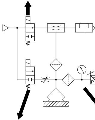
For the release valve, select a 2/3 port valve with a low vacuum specification. Also, use a needle valve to regulate the release flow rate.
