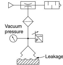
If a considerable amount of leakage occurs between the workpiece and the pad, resulting in incomplete adsorption, or to shorten the adsorption and transfer time, select an ejector nozzle with a larger diameter from the ZH, ZM, ZR, or ZL series.
