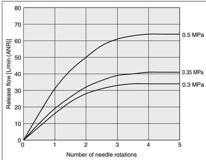
**ZQ□A Low release pressure specification with release pressure supply (PD) port<sup>\*1</sup>**
