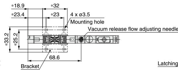
Supply valve (Latching), With release valve
