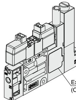
For the port exhaust specification, back pressure may increase depending on the size and length of the piping connected to the exhaust (EXH) port. Ensure that the back pressure does not exceed 0.005 MPa (5 kPa). Do not operate the ejector or apply pressure to the exhaust port with the exhaust port closed. This increases the pressure in the product and can damage the vacuum ejector.
