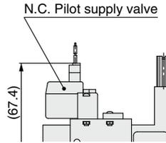
Supply valve (Latching), Without release valve
