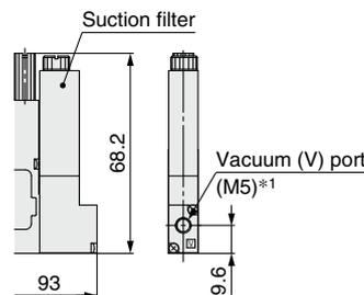
\*1 The pitches of PV, PS, PE, and V ports are determined assuming the use of One-touch fittings.
