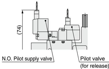
Supply valve (N.C.), With release valve
