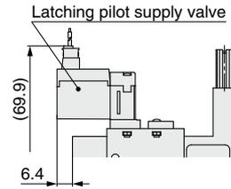
Supply valve (N.O.), With release valve
