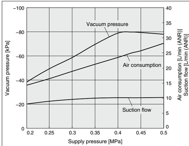
**ZQ07□A: Flow Rate Characteristics** Supply pressure: 0.43 MPa
