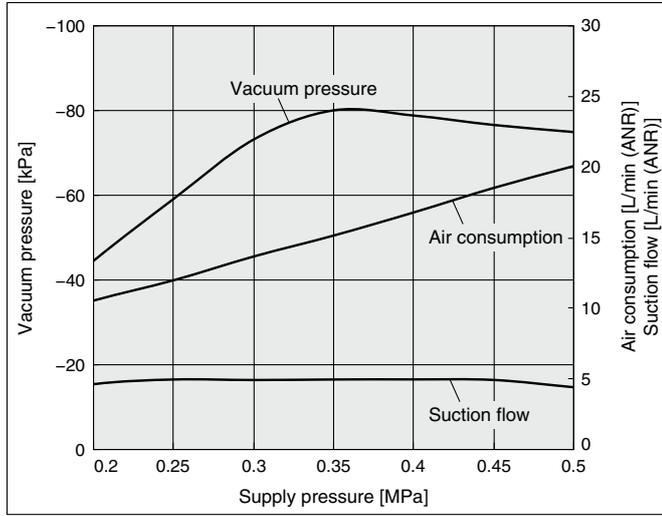
**ZQ05□A: Flow Rate Characteristics** Supply pressure: 0.35 MPa
