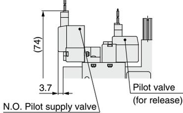
Supply valve (N.C.), With release valve
