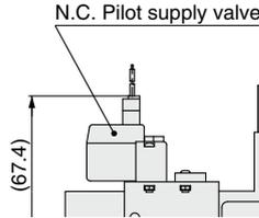
Supply valve (Latching), Without release valve
