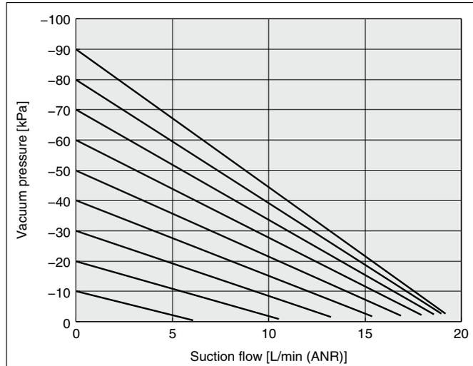
The actual suction flow at the point of suction varies depending on the piping conditions to the vacuum port. (The above graph shows the value when V port is ø6.)
