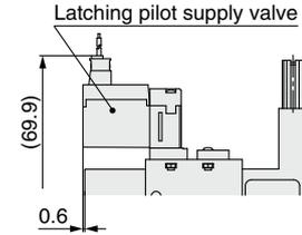
Supply valve (N.O.), With release valve
