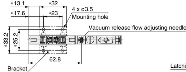
Supply valve (Latching), With release valve
