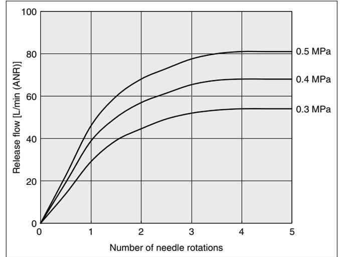
**ZQ□A Without release pressure supply (PD) port (With energy saving switch)**
