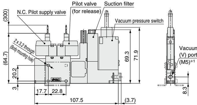
With IO-Link compatible vacuum pressure switch
