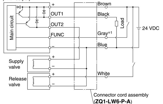
\*1 The gray wire (FUNC) is connected when operating the supply valve by energy saving control (for workpiece adsorption). (For details, please refer to the Operation Manual for the ZQ-ZSV□-□-A series on the SMC website.)
