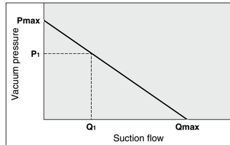
The flow rate characteristics indicate the relationship between the vacuum pressure and the suction flow of the ejector. They also show that when the suction flow changes, the vacuum pressure also changes. In general, this indicates the relationship at the ejector's standard operating pressure. In the graph, **Pmax** indicates the max. vacuum pressure, and **Qmax** indicates the max. suction flow. These are the values that are published as specifications in catalogs, etc.
