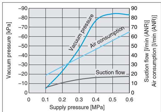
\*1 The exhaust characteristics are different when the vacuum-saving valve (ZP2V-B6-05) is mounted.
