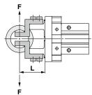
**External Gripping Force** JMHZ2-8D 15 Pressure 0.7 MPa Gripping force [N] -0.6 MPa 10 0.5 MPa 0.4 MPa 0.3 MPa 5 0.2 MPa 0.15 MPa 0 80 100 20 60 0 40 Gripping point L [mm] JMHZ2-12D 30 Pressure 0.7 MPa
