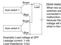
Load voltage at OFF = Leakage current x 2 pcs. x
