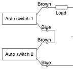
Example) Load voltage at ON Power supply voltage: 24 VDC Internal voltage drop: 4 V
