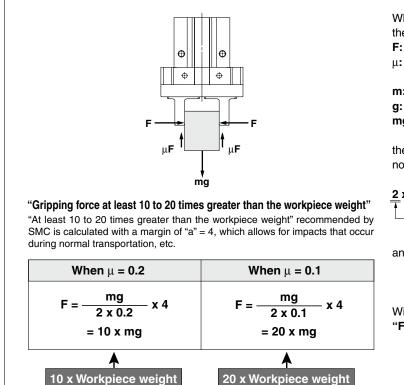
When gripping a workpiece as in the figure to the left, and with the following definitions, F: Gripping force [N]
