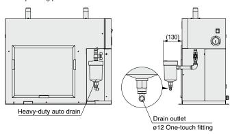
\* The heavy-duty auto drain and piping materials (nipple, elbow) are shipped together with the main body of the air dryer. Customers are required to mount the parts to the air dryer.
