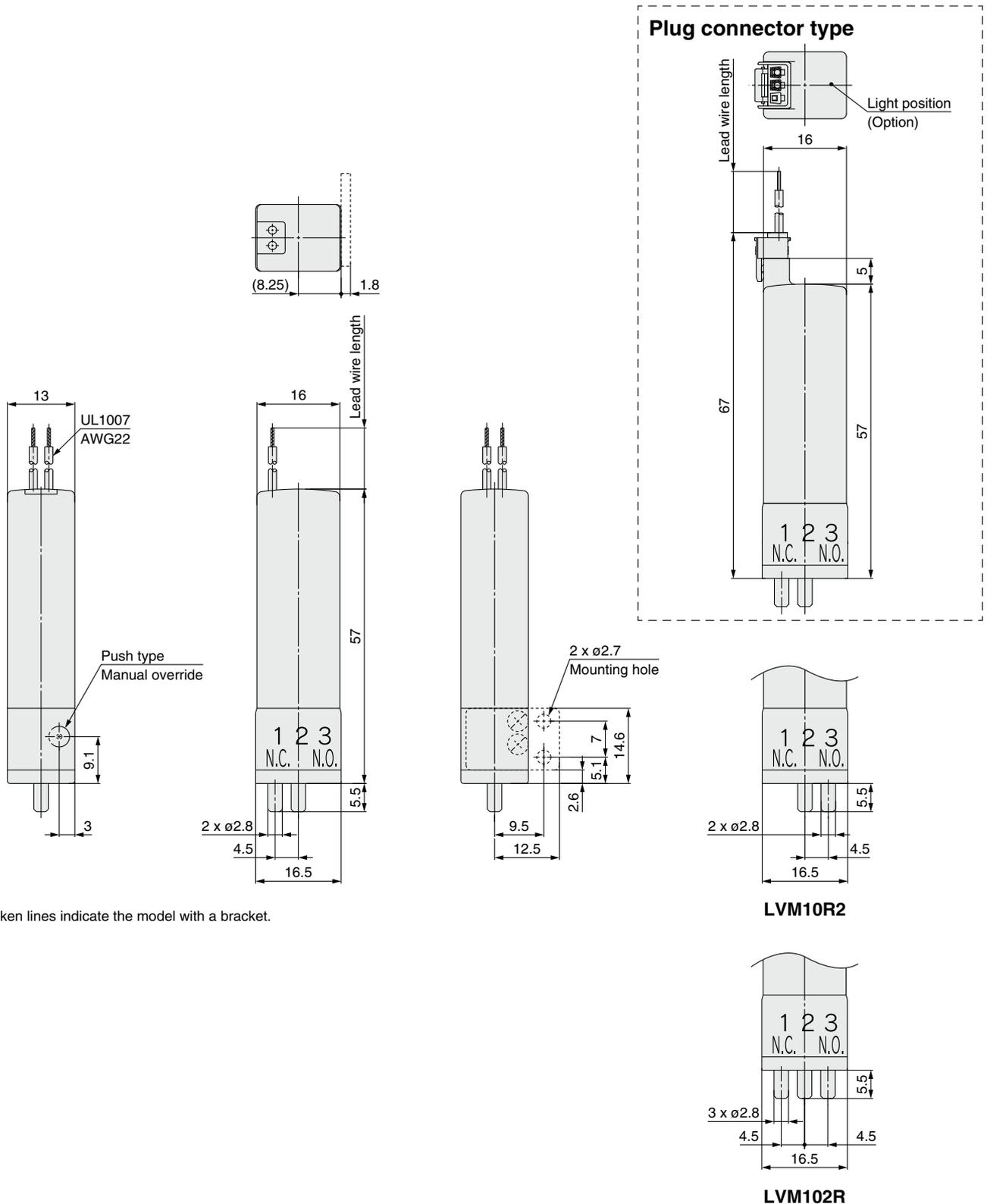
\* The broken lines indicate the model with a bracket.
