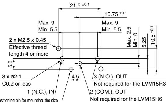
When using a positioning pin for mounting, the size should be  $\phi 1.2$ , and the height should be 2 or less.
