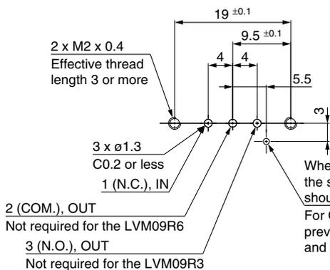
When using a positioning pin for mounting, the size should be ø1, and the height should be 1.5 or less. For Option "P" (With reverse mounting prevention pin), the size should be ø1.7, and the depth should be 2.3 or more.
