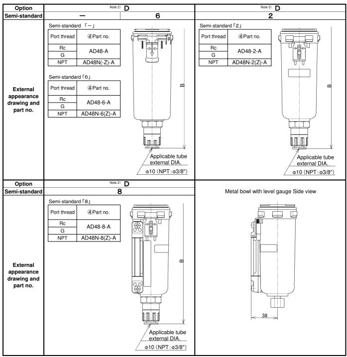
Note 1) B in the table shows the distance from inlet piping centreline to drain port. Refer to "12. DIMENTIONS" (P24).
