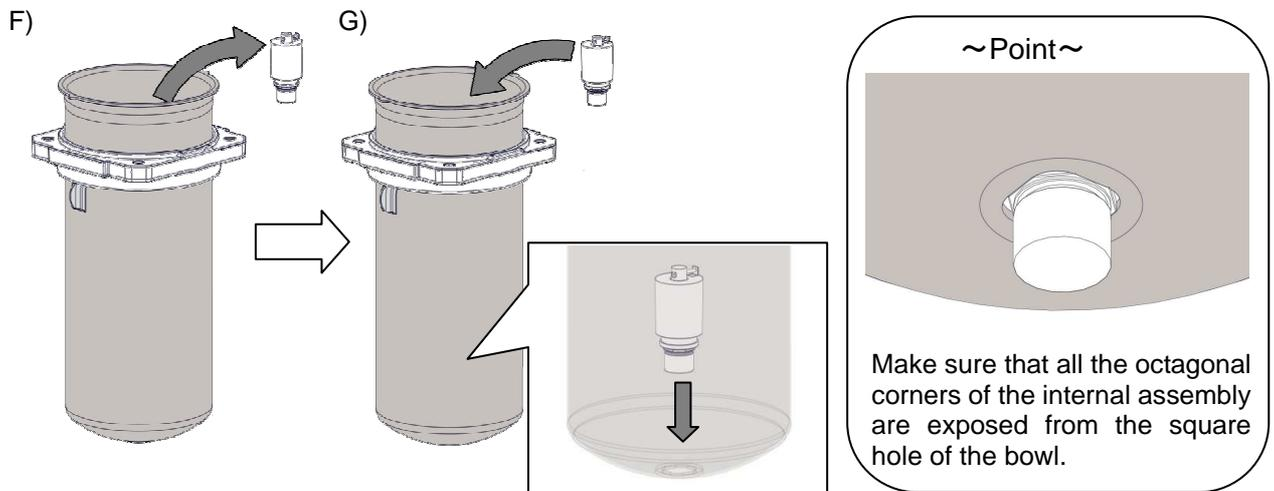
H) Mount the removed drain port spacer.
