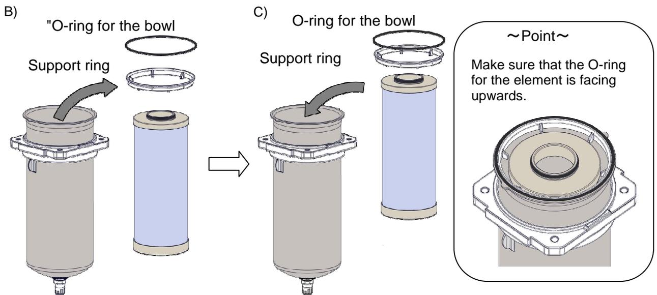
【When it is difficult to insert the new element into the body.】
