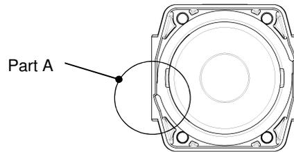
Align the notch groove with the finger of the bowl (Part A).
