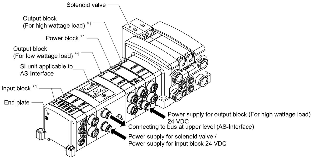
This system connects input/output devices to AS-Interface with reduced wiring. AS-Interface communicates with the input/output devices via the SI unit.
