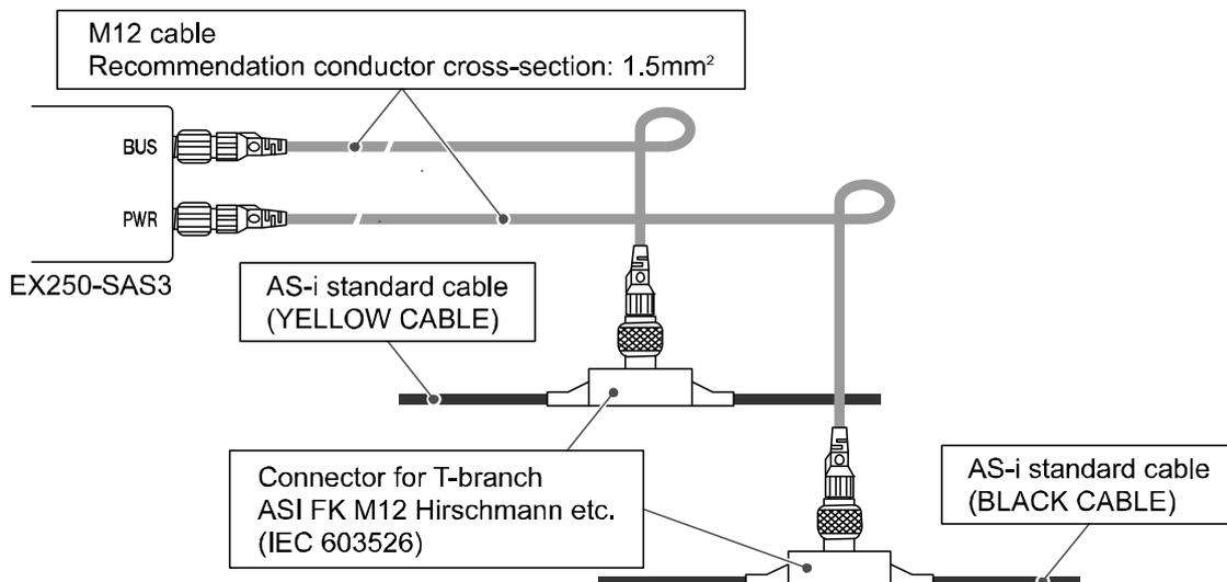
The M12 cable, AS-i standard cable and connector for T-branch are not supplied by SMC. Contact each manufacturer for the catalogue details etc.
