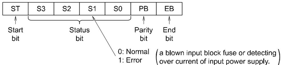
It is possible to confirm the peripheral fault error only by status register on the ADDR1 side for EX250-SAS3/-SAS7 which occupy 2 slaves.
