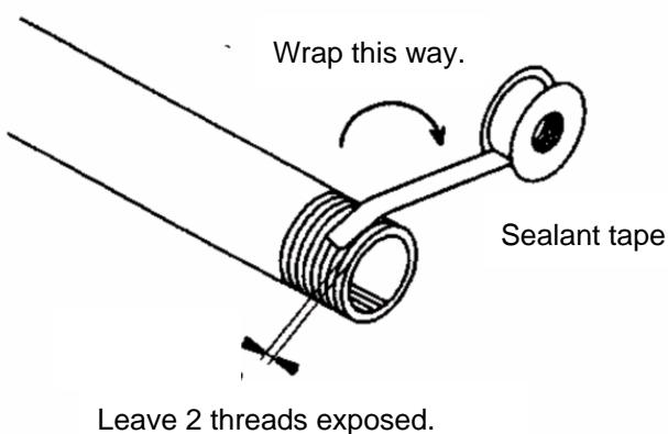
**Fig. 2 Sealant tape**
