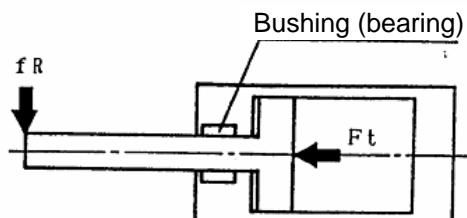
Fig. 1 Allowable lateral load applied to rod end
