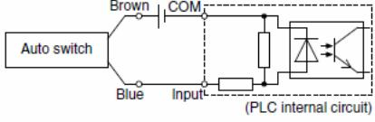
Connect according to the applicable PLC input specifications, as the connection method will vary depending on the PLC input specifications.
