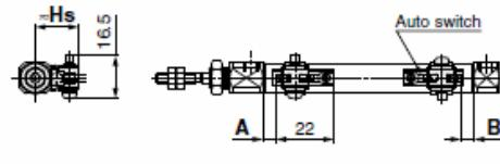
A and B are the dimensions from the end of the head cover/rod cover to the end of the auto switch.
