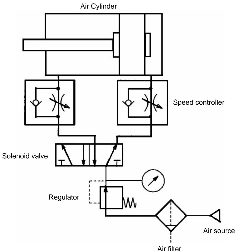
**Fig.3 Basic Circuit**
