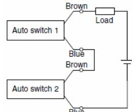
When two auto switches are connected in series, malfunction may occur because the load voltage will decrease in the ON state. The indicator lights will light up when both of the auto switches are in the ON state.
