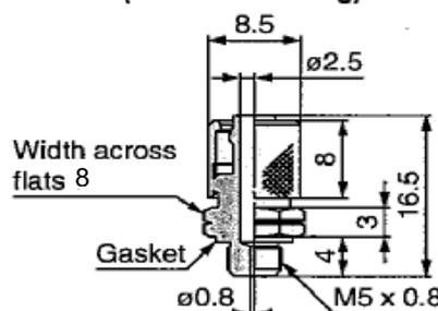
In addition to the above fittings and hose nipples, the below fittings can also be attached to the cylinder. When using the below fittings be sure to provide a speed controller after adjusting it to 500 mm/sec or less.
