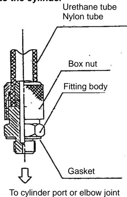
A hose nipple consists of two parts: a fitting body and a box nut.
