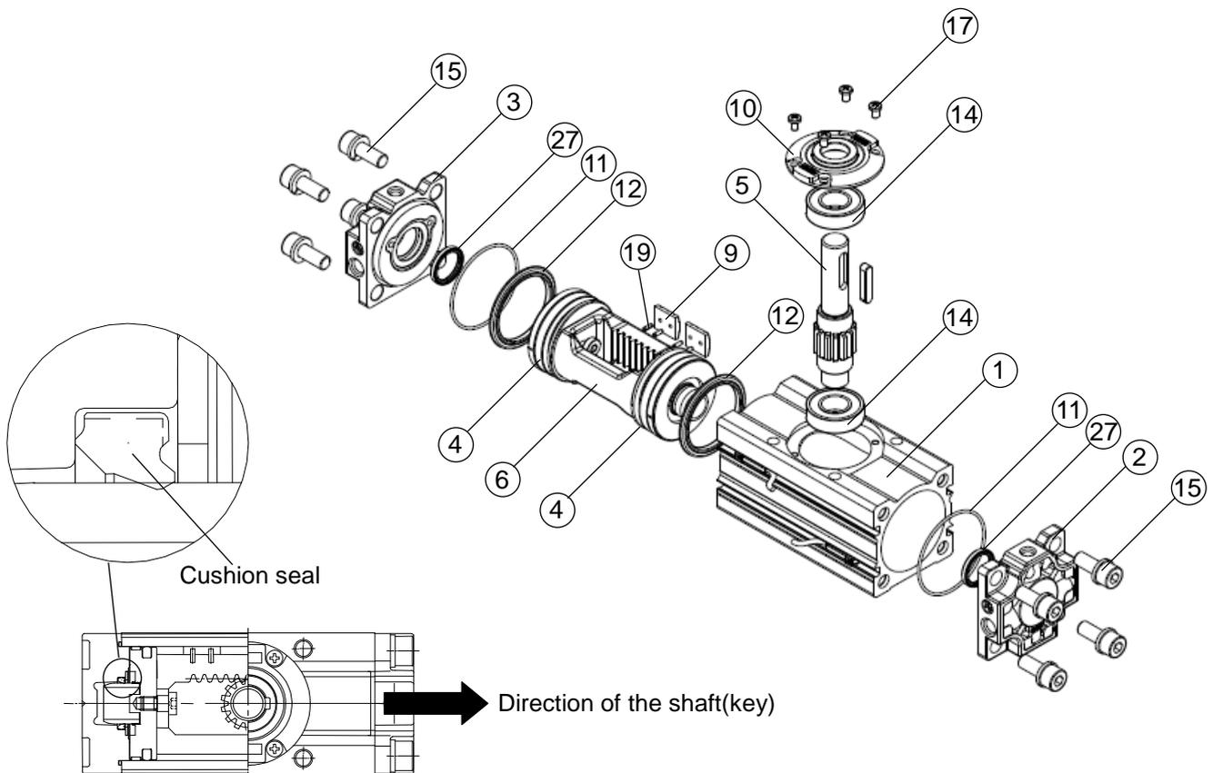
Fig. (18) Direction of assembly of the shaft
