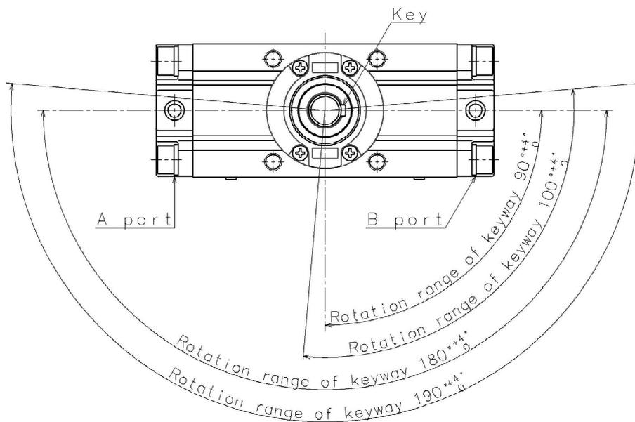
Fig. (2) Rotation range of shaft keyway (size 50 to 100)
