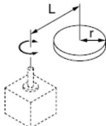
$I = K + m \cdot L^2$ <p>K: Moment of inertia around the load center of gravity<br/>4. Round plate <math>K = m \cdot \frac{r^2}{2}</math></p>                                                                                             |
