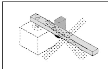
The external stopper becomes a fulcrum, resulting in the load's inertia force being applied to the shaft as a bending moment.
