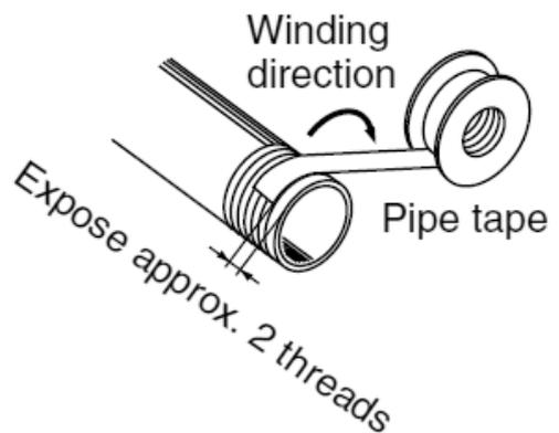
Fig. (11) Wrapping of pipe tape
