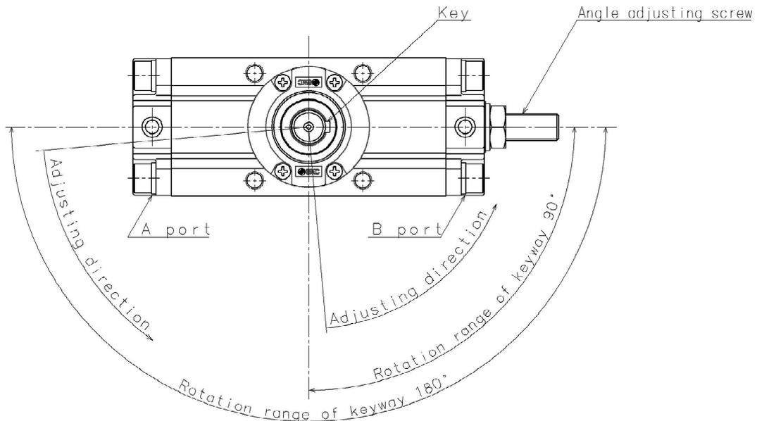
Fig. (3) Rotation range of shaft keyway (angle adjustable type)
