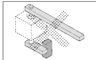
If an external stopper is installed on the shaft side which is opposite of the load, the inertia force generated by the load is applied directly to the shaft.
