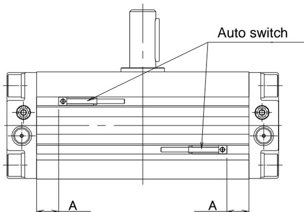
Fig. (14) Proper auto switch mounting position
