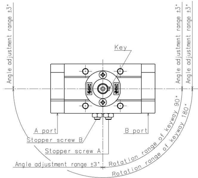
Stopper screw A : For end adjustment in clockwise direction
