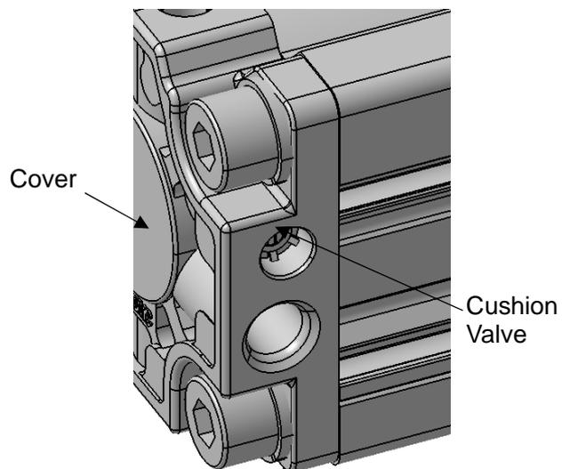
Fig. (5) How to Adjust the Air cushion
