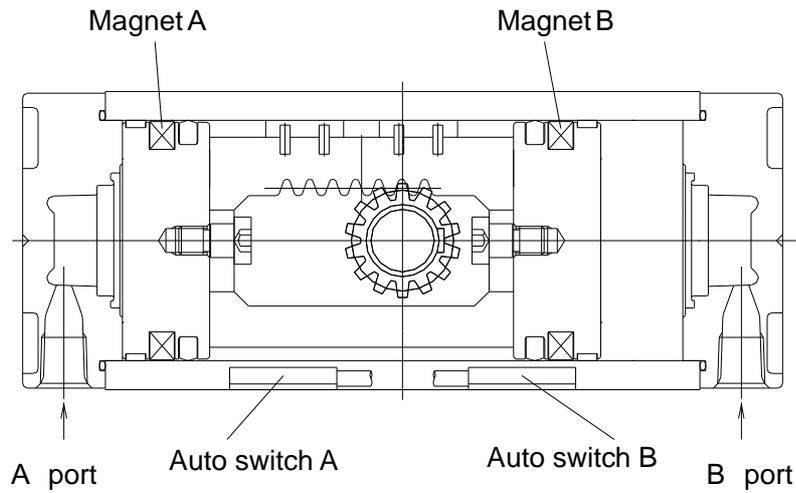
Fig. (16) Auto switch operation principle
