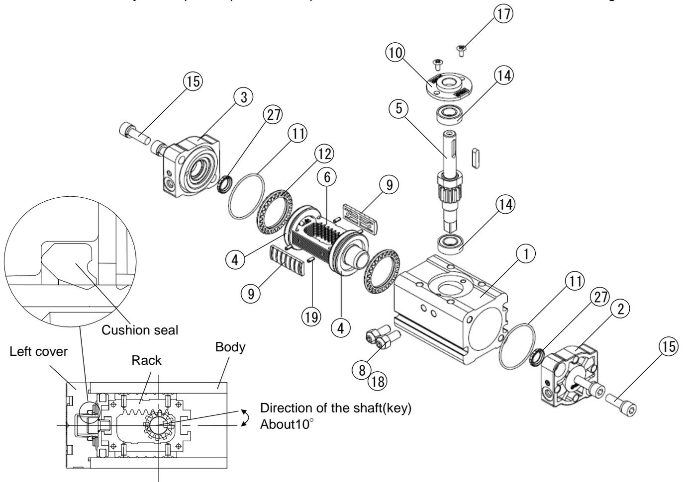
Fig. (17) Direction of assembly of the shaft
