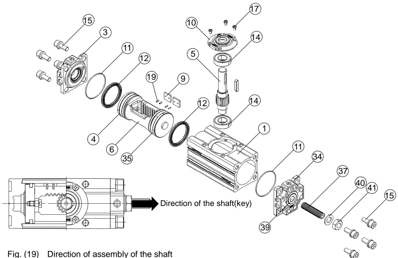
Fig. (19) Direction of assembly of the shaft
