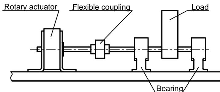
Fig. (9) Flexible coupling
