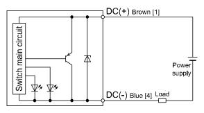
Note: The number marked on each lead wire color shows the pin number of pre-wired connector.
