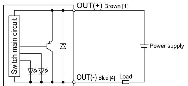
\*: The number marked on each lead wire color shows the pin number of pre-wired connector.
