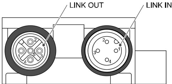
LINK IN: M12 4-pin plug, A-coded
