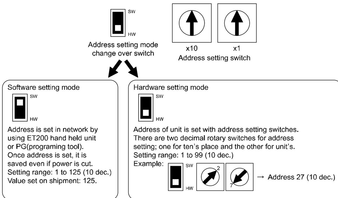
\*: When software setting mode is selected, address setting switches are not effectual. Moreover, software setting mode and hardware setting mode differ in ID numbers of units. (See "I/O Configuration" (page 19) for details.)
