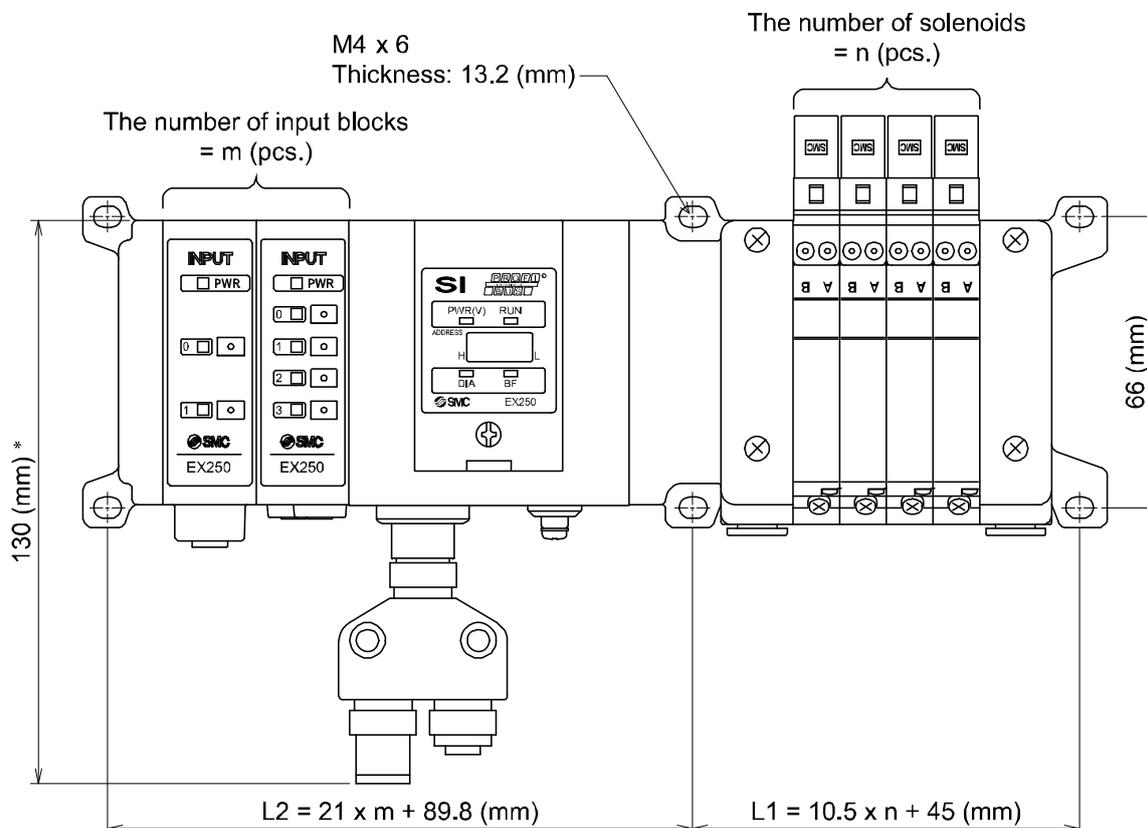
\*: The size when connecting Bus Tee with the SI unit directly.
