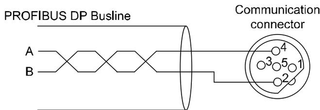
Cable: Shielded twisted pair cable (Type-A cable)
