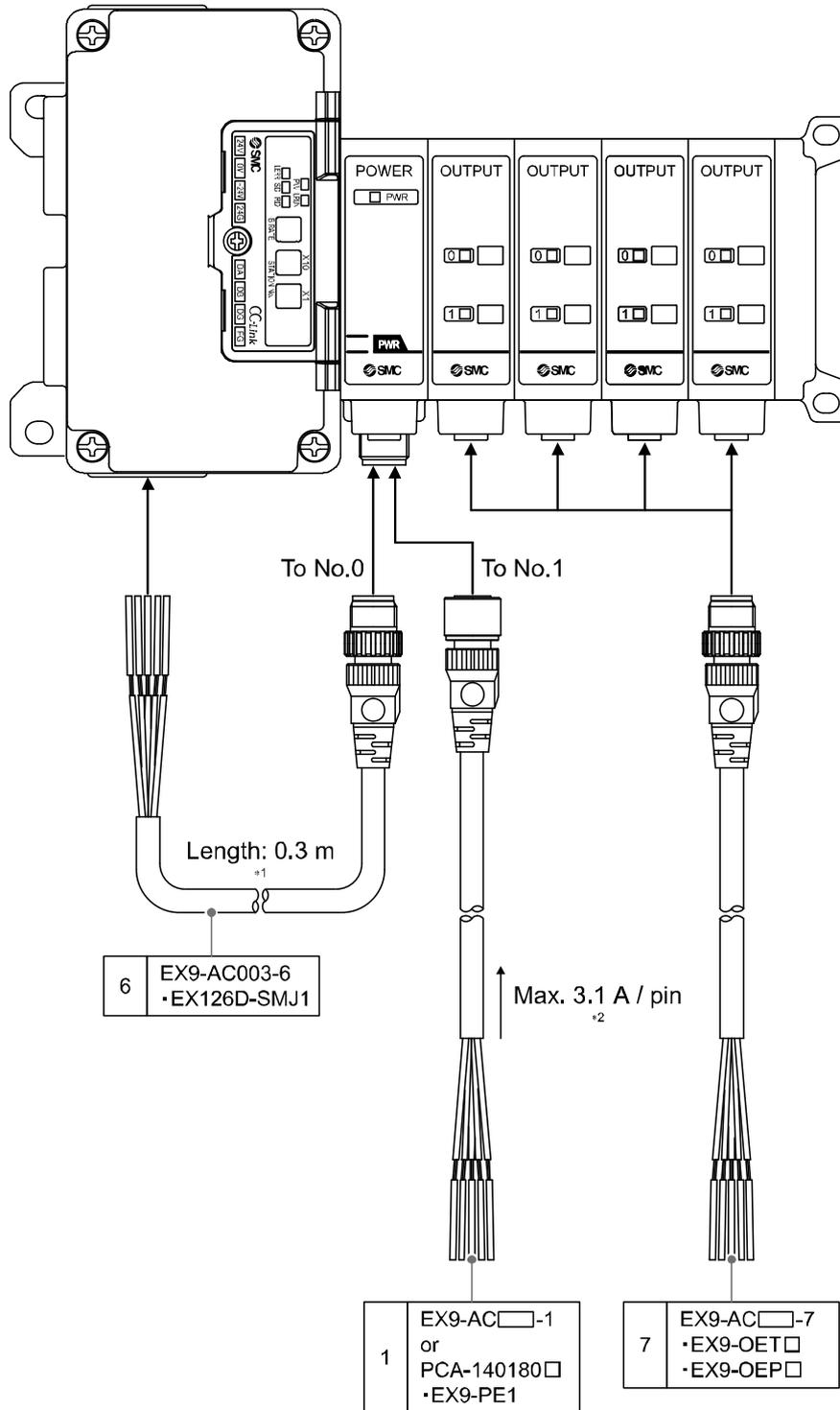
\*1: This cable is a bypass cable used for the layout where the Power block is located to the right of the SI unit.
