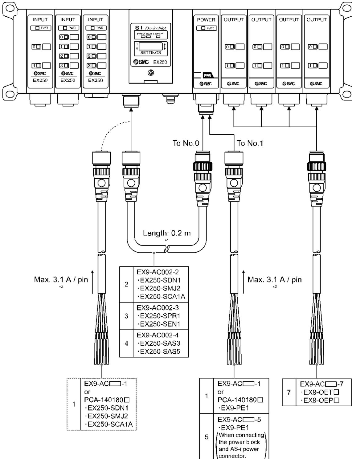
\*1: This cable is a bypass cable used for the layout where the Power block is located to the right of the SI unit.
