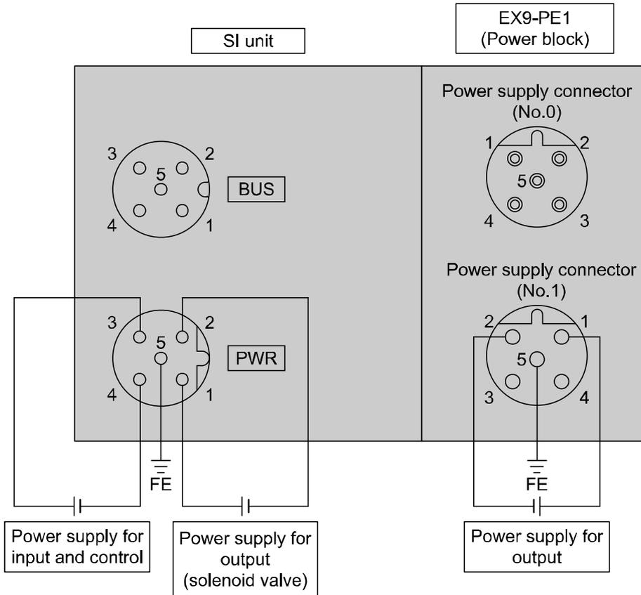
•Connecting the power supply from the Power block (EX9-PE1) to the SI unit.
