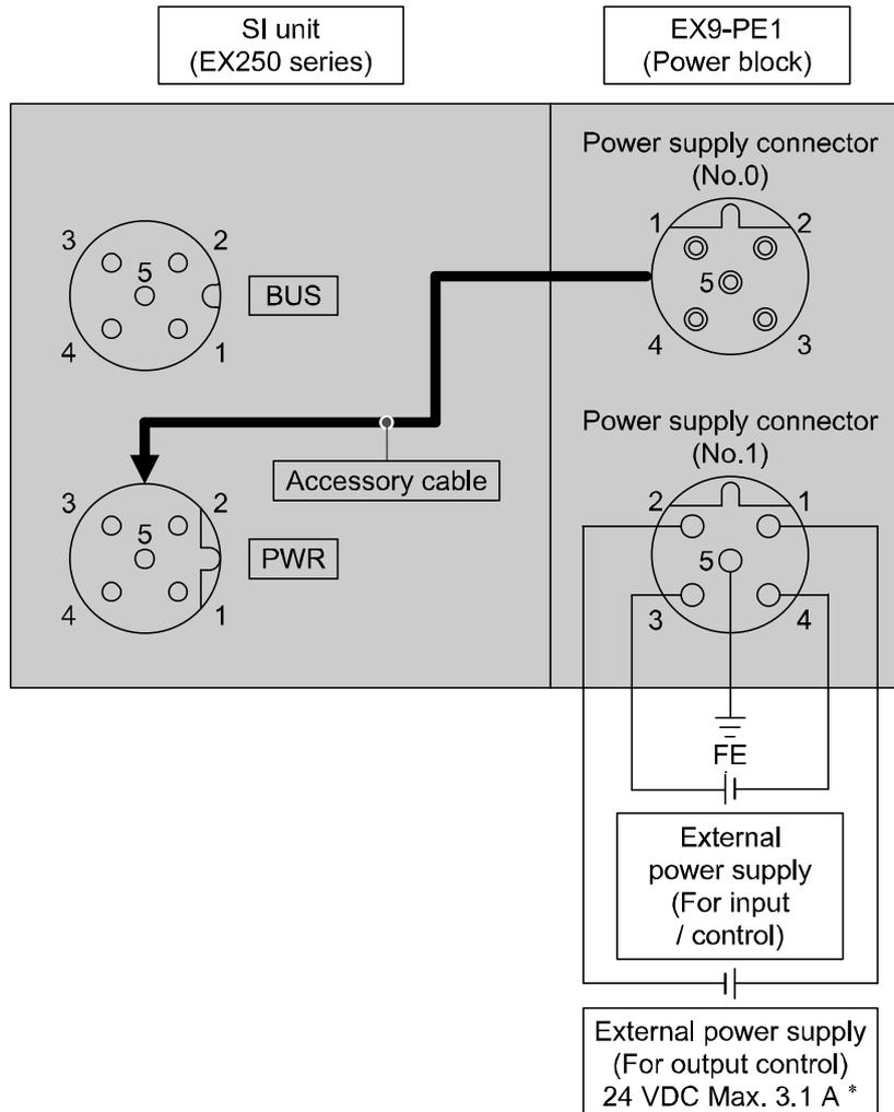
\*: When maximum supply current is 3.0 to 3.1 A, keep the ambient temperature at 40 °C or less and do not bundle the cable.
