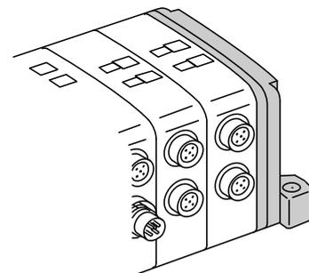
(5) Bracket plate for mounting EX260 series Output block and DIN rail mounting bracket
