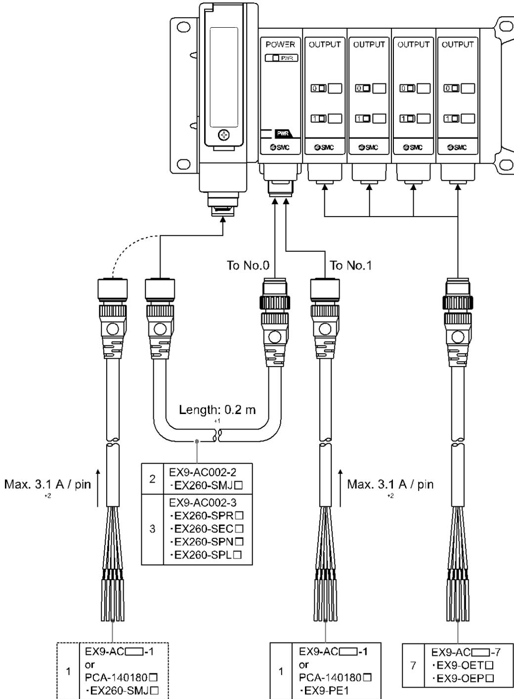
\*1: This cable is a bypass cable used for the layout where the Power block is located to the right of the SI unit.
