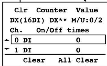
3. The counter value of each channel of the unit selected is displayed. Select the channel with the **▲** and **▼** buttons. (If all the channels are cleared, this operation is not necessary.)
