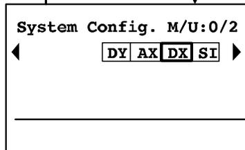
2. Select the unit with the **◀** and **▶** buttons and press the **ENTER** button. It is not possible to select the analog unit.
