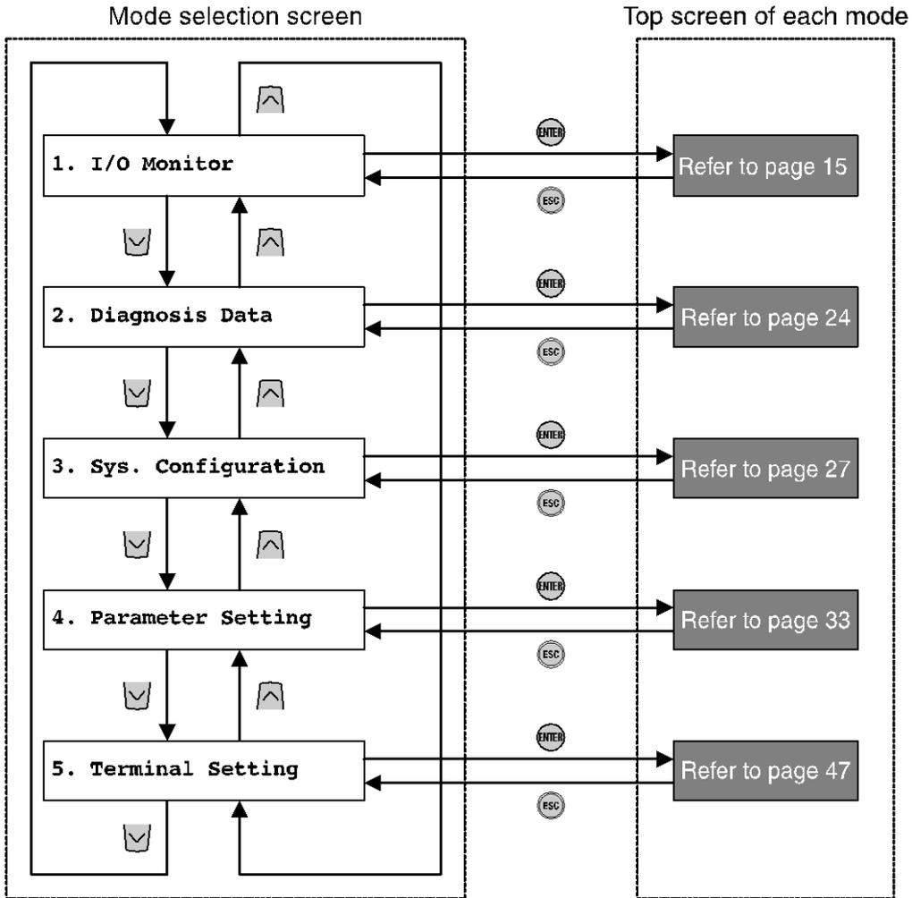
\*: When each button is pressed, the mode shifts in the direction indicated by the arrow.
