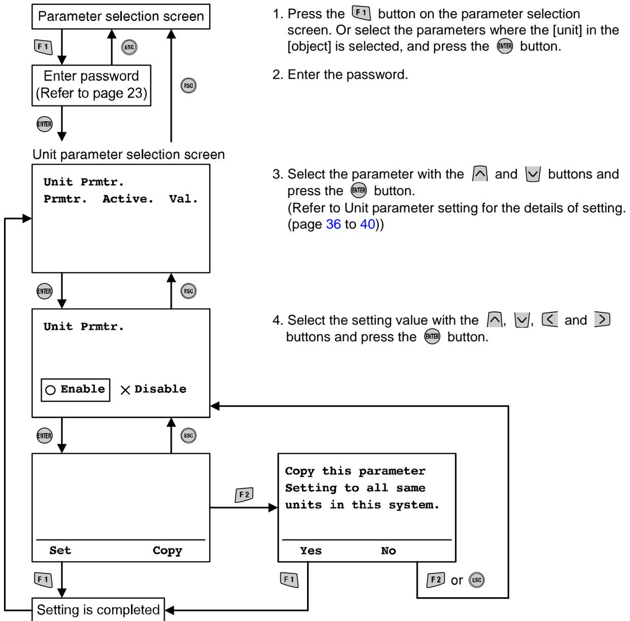
1. Press the **F1** button on the parameter selection screen. Or select the parameters where the [unit] in the [object] is selected, and press the **ENTER** button.
