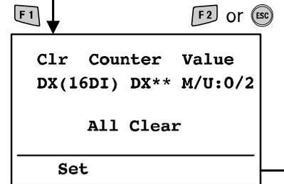
5. Press the **F1** button. The counter values of the channel selected or all of the channels are cleared.
