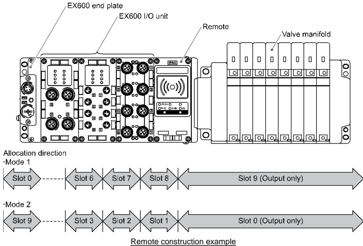
The remote is positioned at the center of the remote, so that the EX600 I/O units can be connected to the left side of the remote and the valve manifold can be connected to the right side of the remote, similar to the base.
