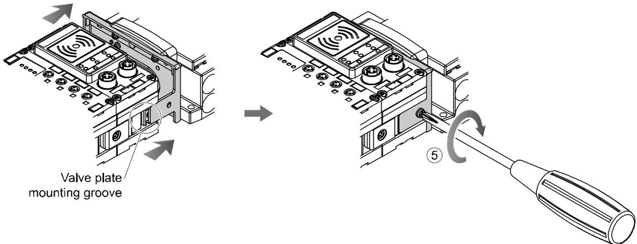
(6) When valve manifold is not connected.
