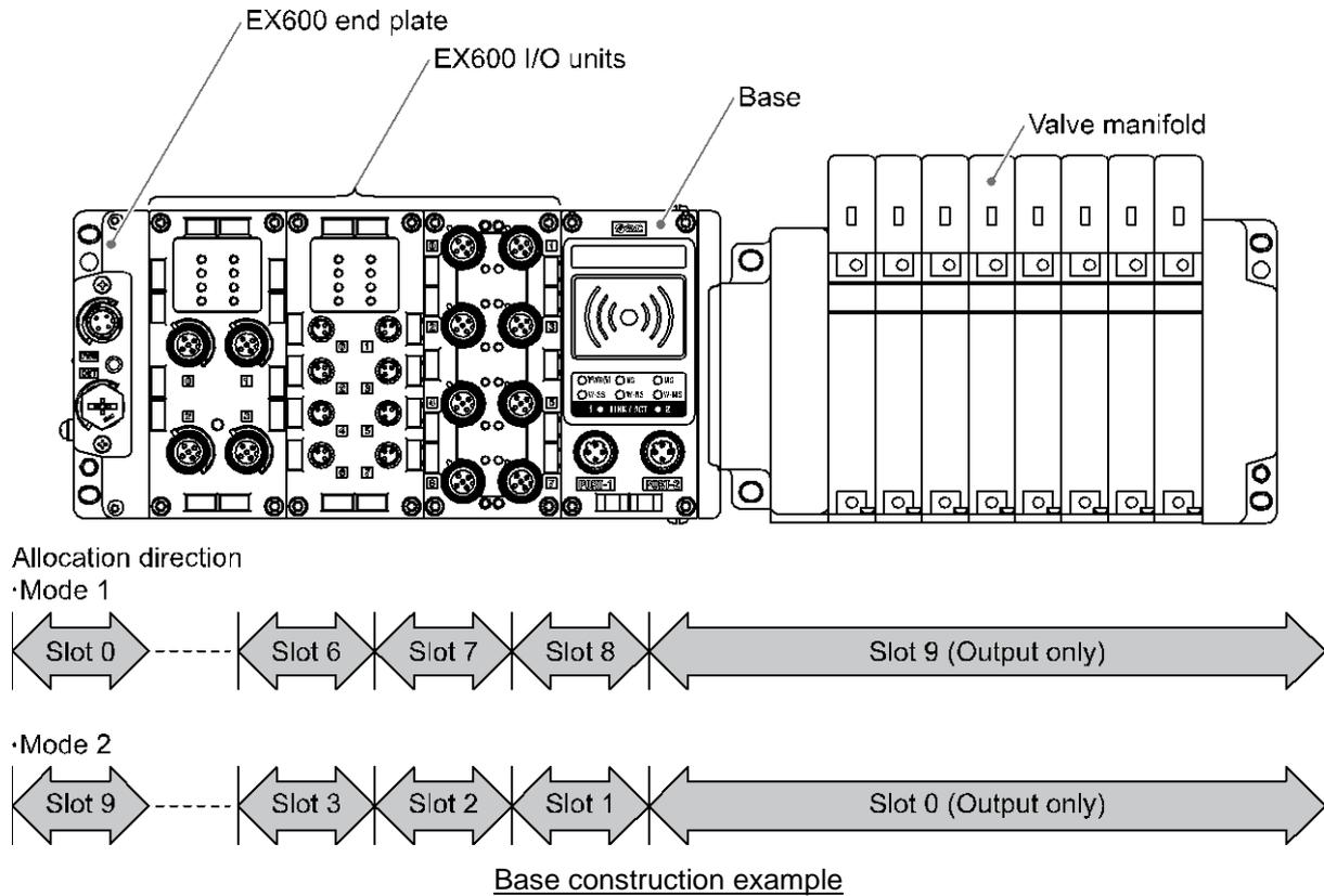
The **base** is positioned at the center of the **base**, so that the EX600 I/O units can be connected to the left side of the base and the valve manifold can be connected to the right side of the base. Refer to the SMC catalogue for the EX600 series serial transmission system for the wiring method. [http://ca01.smcworld.com/catalog/BEST-5-1-en/mpv/e02-24-ex600/pageview.html#page\\_num=C1](http://ca01.smcworld.com/catalog/BEST-5-1-en/mpv/e02-24-ex600/pageview.html#page_num=C1)
