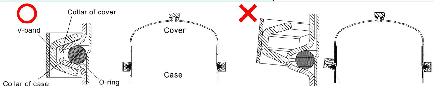
Fig. (a) Correct mounting of V-band
