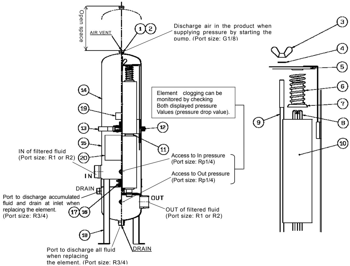
**Fig. 1 Description of parts and functions**
