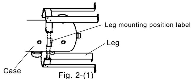
(2) Close the legs, and mount the hexagon head bolts and nuts, which are delivered together with the product, onto the bolt mounting holes on the legs and tighten them at 12.5 Nm.
