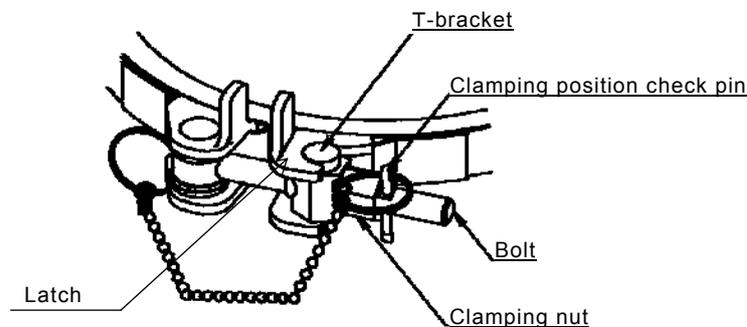
Fig. (c) V band tightening
