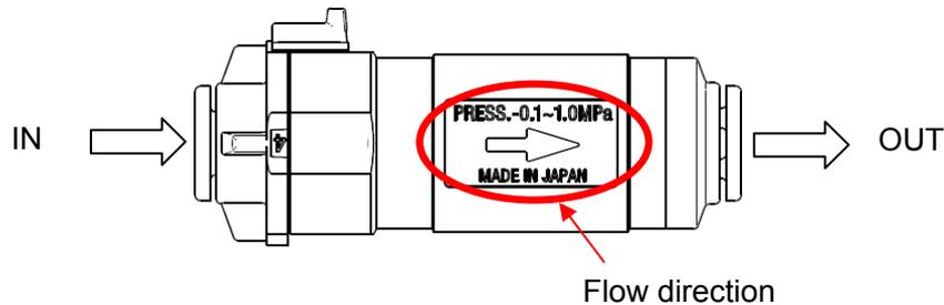
Note) When replacing the element, ensure that there is enough space for removing the cover (IN side).
