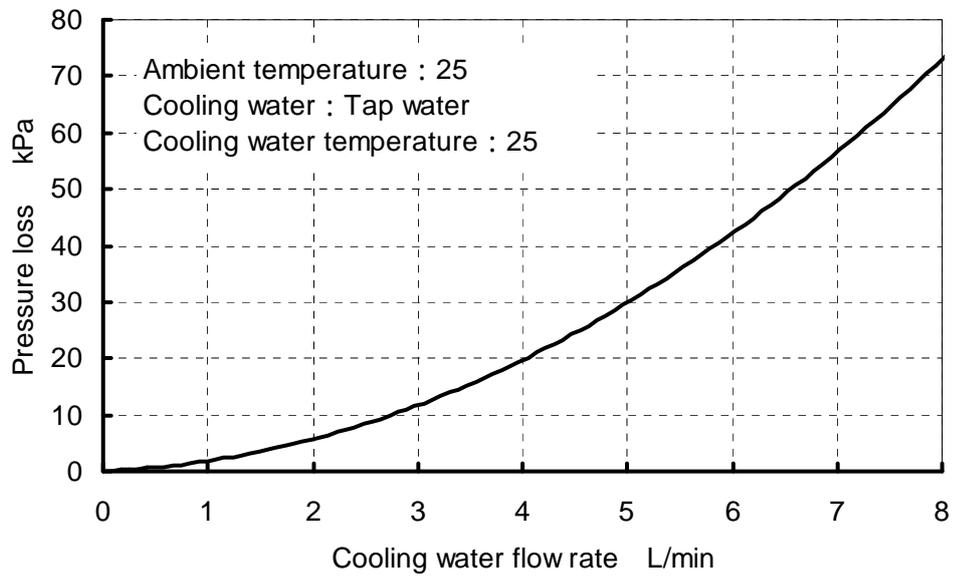
Fig. 7-6 Radiating water pressure loss
