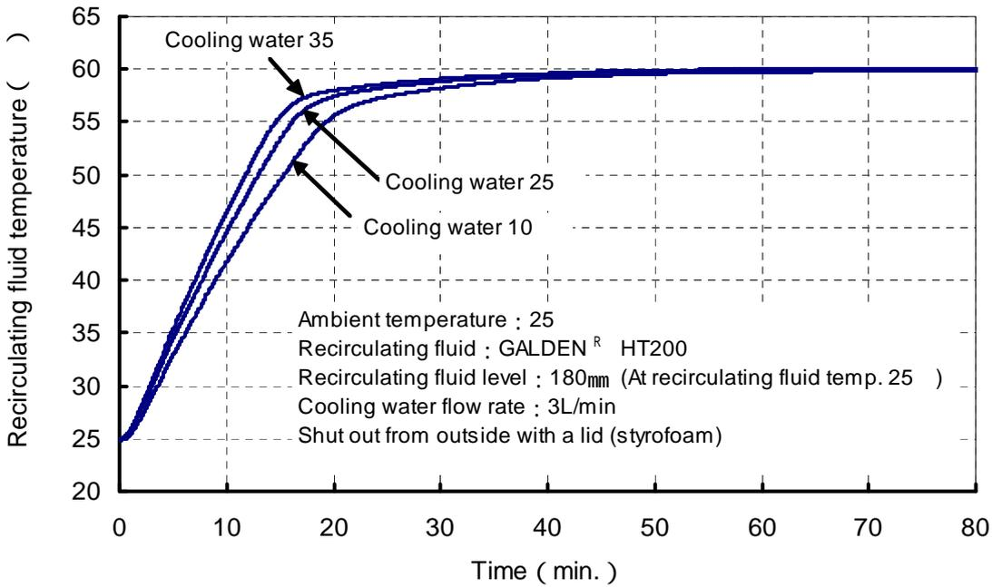
Fig. 7-5 Heating capacity
