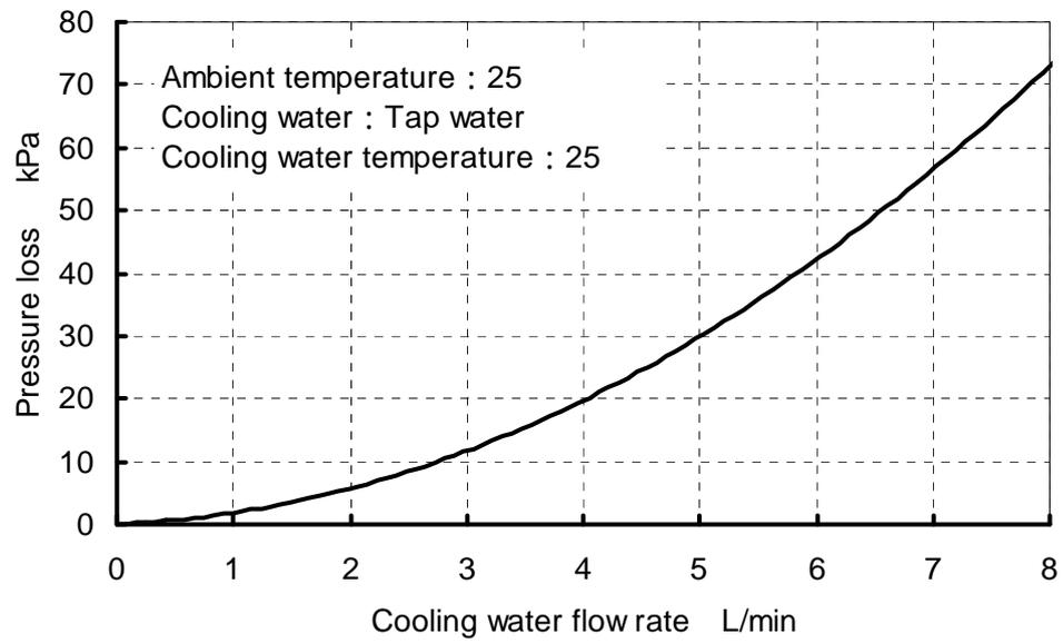
Fig. 7-6 Radiating water pressure loss
