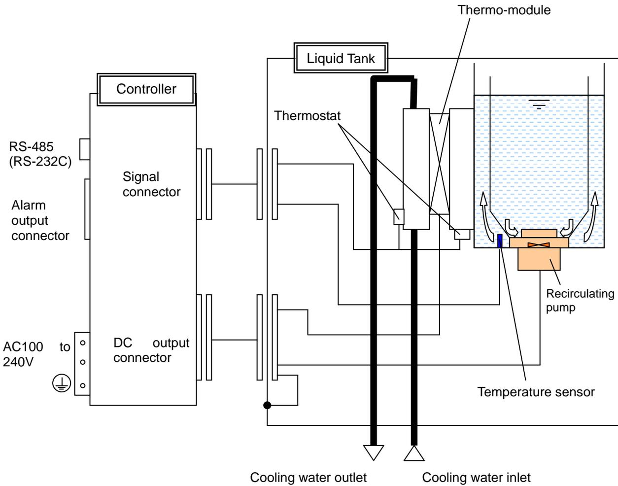
Fig. 3-3 Operation principle
