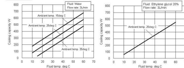
\*Cooling capacity decrease about 20W when high head pump option selected.
