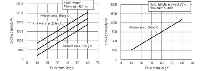
\*Cooling capacity decrease about 50W when high head pump option selected.
