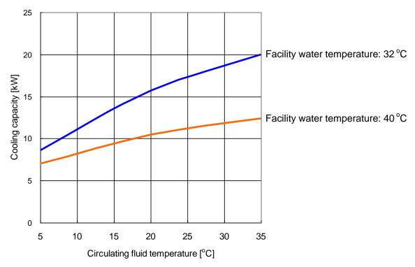
Fig. 8-13: Cooling Capacity (HRSH150-W\*-20/40-\*)
