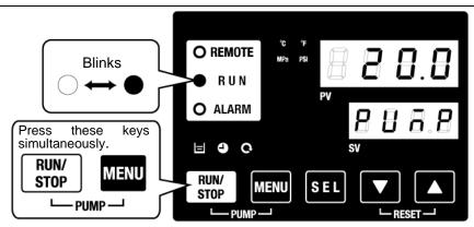
Fig. 4-4 Individual operation of the pump
