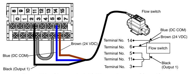
Fig. 3-12 Wiring of the external switch (NPN open collector output) (example)
