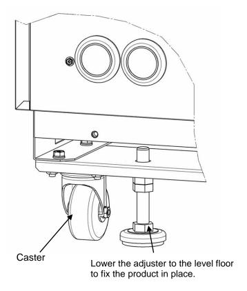
Fig. 3-5 Installation by adjuster foot
