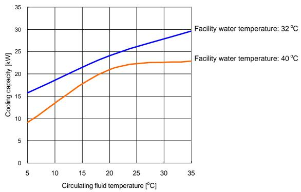
Fig. 8-15: Cooling Capacity (HRSH250-W\*-20/40-\*)
