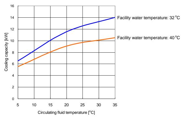
Fig. 8-12: Cooling Capacity (HRSH100-W\*-20-\*)
