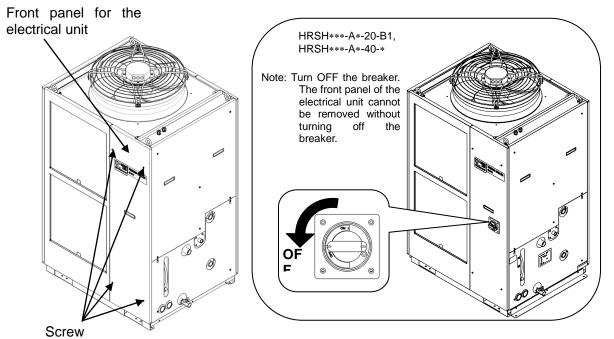
Fig. 6-1: Removal of the front panel of the electrical unit
