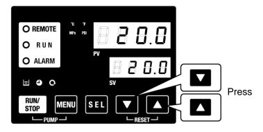
Fig. 4-3 Setting of circulating fluid temperature
