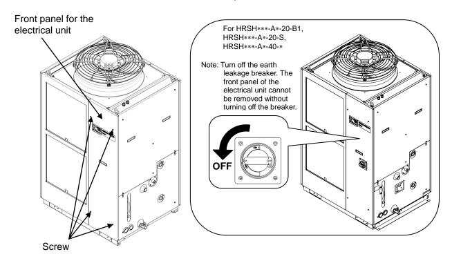
Fig. 3-6 Remove the front panel for the electrical unit (This drawing shows air cooled type.)
