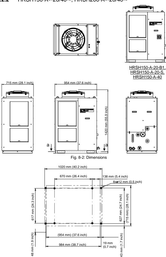
Dimensions for the positions of the anchor bolts (View a-a)
