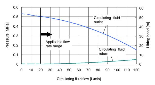
Fig. 8-16: Pump capacity (HRSH100-A\*-20/40-\*, HRSH100-W\*-20/40-\*)
