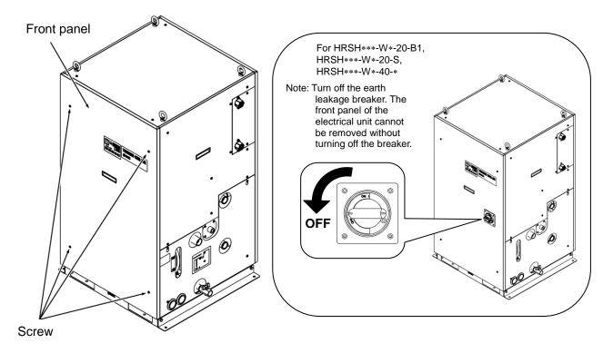
Fig. 3-7 Remove the front panel for the electrical unit (This drawing shows water cooled type.)
