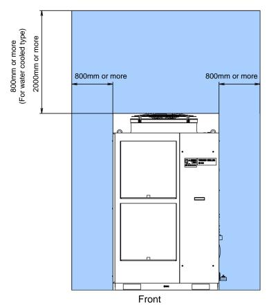
Fig. 3-3 Installation space (This drawing shows "HRSH250-A-20".)
