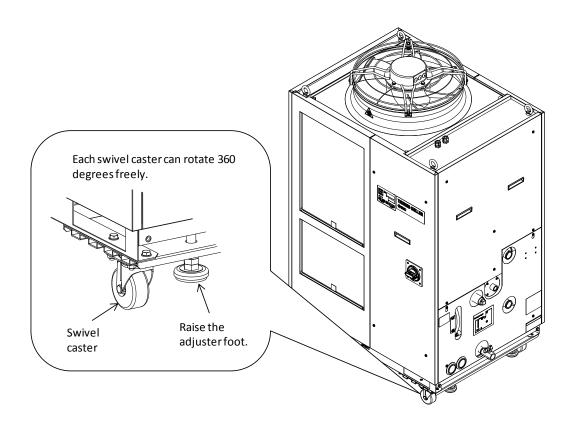
Fig. 3-2 Transportation using casters (This drawing shows "HRSH250-A-20".)
