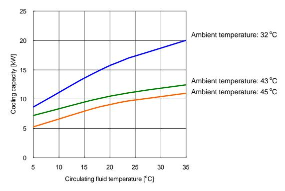
Fig. 8-8: Cooling Capacity (HRSH150-A\*-20/40-\*)
