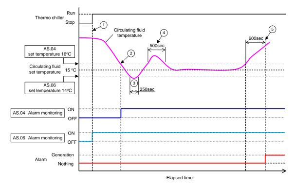
Fig 5.22-1: Alarm generation timing
