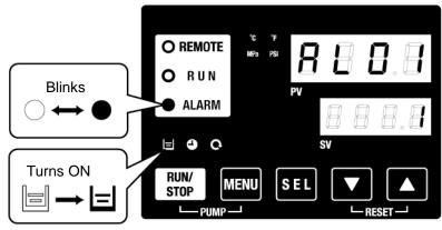
Fig. 4-5 Low level in tank" alarm
