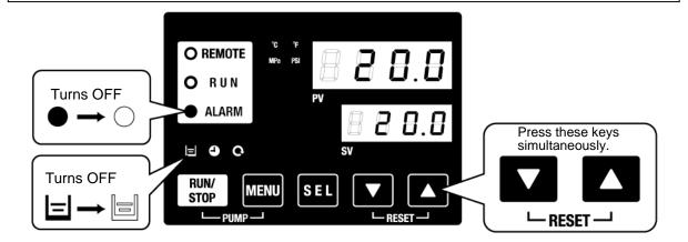
Fig. 4-7 Reset of the alarm
