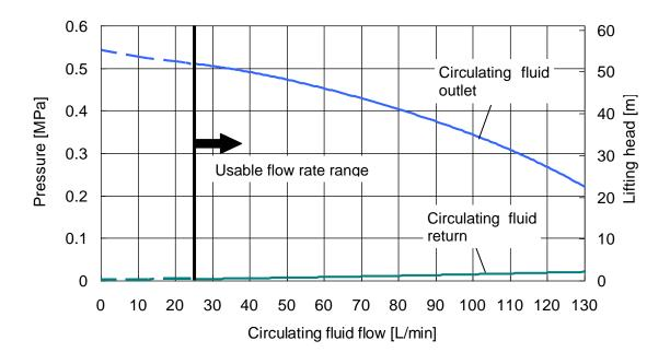
Fig. 8-17: Pump capacity (HRSH150/200-A\*-20/40-\*, HRSH150/200/250-W\*-20/40-\*)
