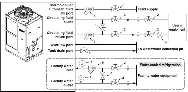
Fig. 3-18 Recommended piping circuit
