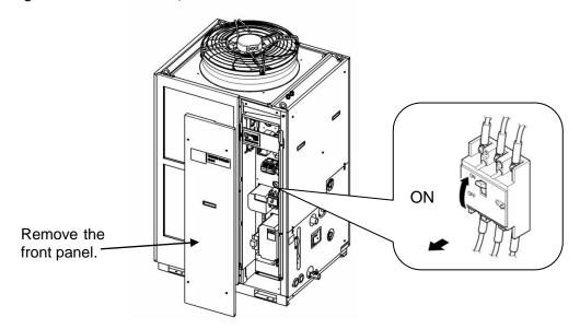
Fig. 4-1 Position of the earth leakage breaker (This drawing shows "HRSH250-A-20-B".)
