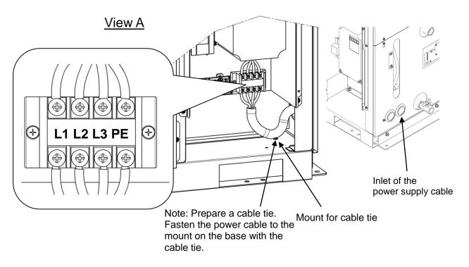
Fig. 3-10 Wiring of power supply cable
