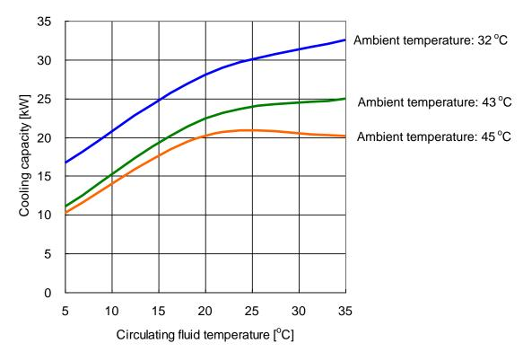
Fig. 8-11: Cooling Capacity (HRSH300-A\*-20/40-\*)
