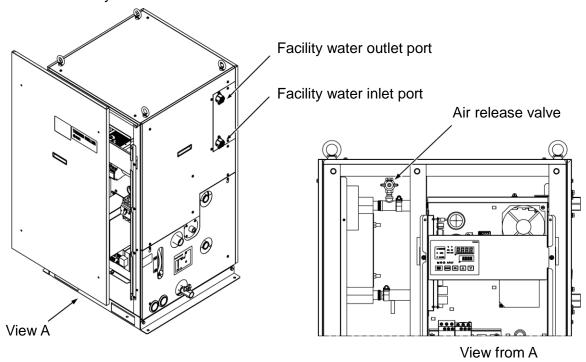
Fig. 7-3: Discharge of the facility water
