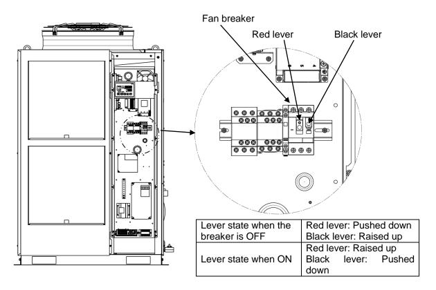
Fig. 6-3: Location and state of the fan breaker
