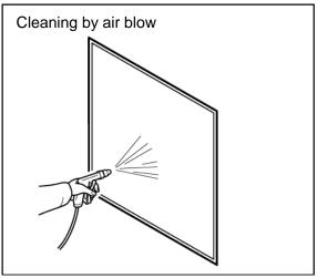
Fig. 7-2: Cleaning of the dust-proof filter
