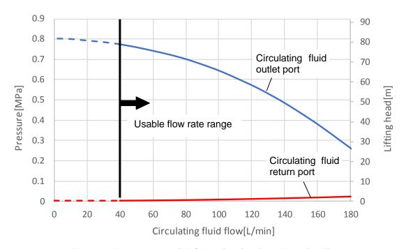
Fig. 8-19: Pump capacity (HRSH100/150/200/250-W\*-20/40-T)
