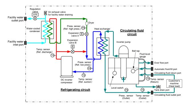
Fig. 8-6: Flow Diagram (HRSH\*\*\*-W\*-20/40-\*)
