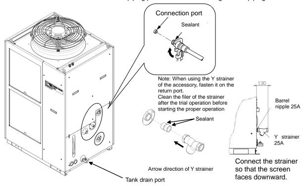
Fig. 3-16 Tightening of piping
