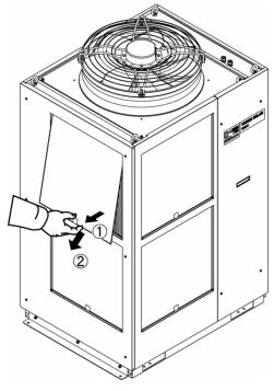
Fig. 7-1: Removal of the dust-proof filter
