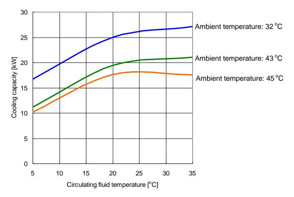
Fig. 8-10: Cooling Capacity (HRSH250-A\*-20/40-\*)
