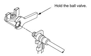
Fig. 3-17 Connection to the drain port
