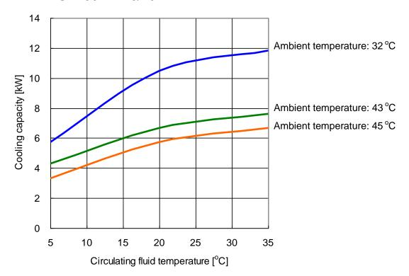
Fig. 8-7: Cooling Capacity (HRSH100-A\*-20/40-\*)
