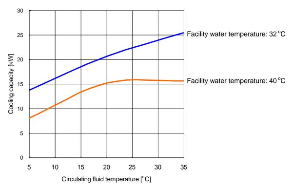
Fig. 8-14: Cooling Capacity (HRSH200-W\*-20/40-\*)
