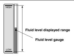
Fig. 3-19 Fluid level gauge
