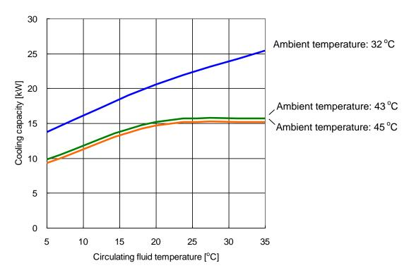
Fig. 8-9: Cooling Capacity (HRSH200-A\*-20/40-\*)
