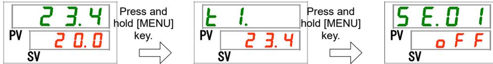
Setting/Checking: Temperature unit
