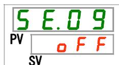
3. Select operation restoration function after power failure with [▲] key or [▼] key, and press [SEL] key to enter.
