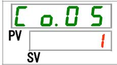
**10.** Set slave addresses (MODBUS) with [▲] key or [▼] key, and press [SEL] key to enter.
