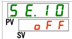
3. Select anti-freezing function with [▲] key or [▼] key, and press [SEL] key to enter.
