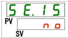
**3.** Select  with [▲] key or [▼] key, and press [SEL] key to enter. Select  and press [SEL] key to enter, and the accumulated operating time of the pump will be reset. The display returns to the main menu.
