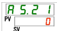
**31.** Set temperature alarm monitoring method with [▲] key or [▼] key, and press [SEL] key to enter.
