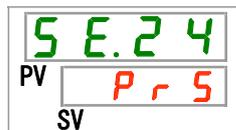
3. Select a pump operation mode with [▲] key or [▼] key, and press [SEL] key to confirm.
