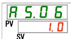
**11.** Set the threshold detecting temperature for "Circulating fluid discharge temp. drop" alarm generation with [▲] key or [▼] key, and press [SEL] key to enter.
