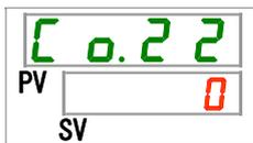
**44.** Set threshold time for the contact input signal 2 OFF detection timer with [▲] key or [▼] key, and press [SEL] key to enter.
