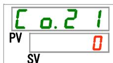
**42.** Set time delay for the contact input signal 2 delay timer for reading with [▲] key or [▼] key, and press [SEL] key to enter.
