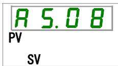
**15.** Set the threshold detection pressure for "Circulating fluid discharge pressure rise" alarm generation with [▲] key or [▼] key, and press [SEL] key to enter.
