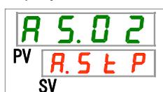
3. Set the product operation when "Low level in tank" alarm is generated with [▲] key or [▼] key, and press [SEL] key to enter.
