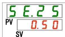
5. Set circulating fluid discharge pressure with [▲] key or [▼] key, and press [SEL] key to enter.
