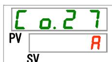
**54.** Set the operation type of the contact output signal 2 with [▲] key or [▼] key, and press [SEL] key to enter.
