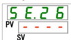
7. Set circulating fluid discharge pressure with [▲] key or [▼] key, and press [SEL] key to enter.
