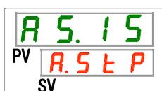
**29.** Set the product operation when "DC line fuse cut" alarm is generated with [▲] key or [▼] key, and press [SEL] key to enter.
