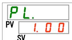
Checking: Accumulated operating time of the pump
