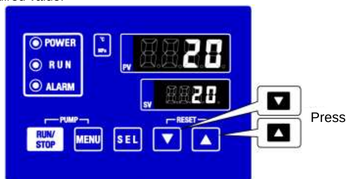
Fig. 4.2-2 Setting of circulating fluid temperature
