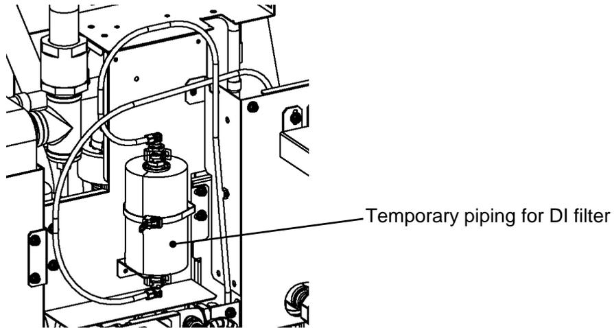
Fig. 7-4 Temporary pipe installation for DI filter
