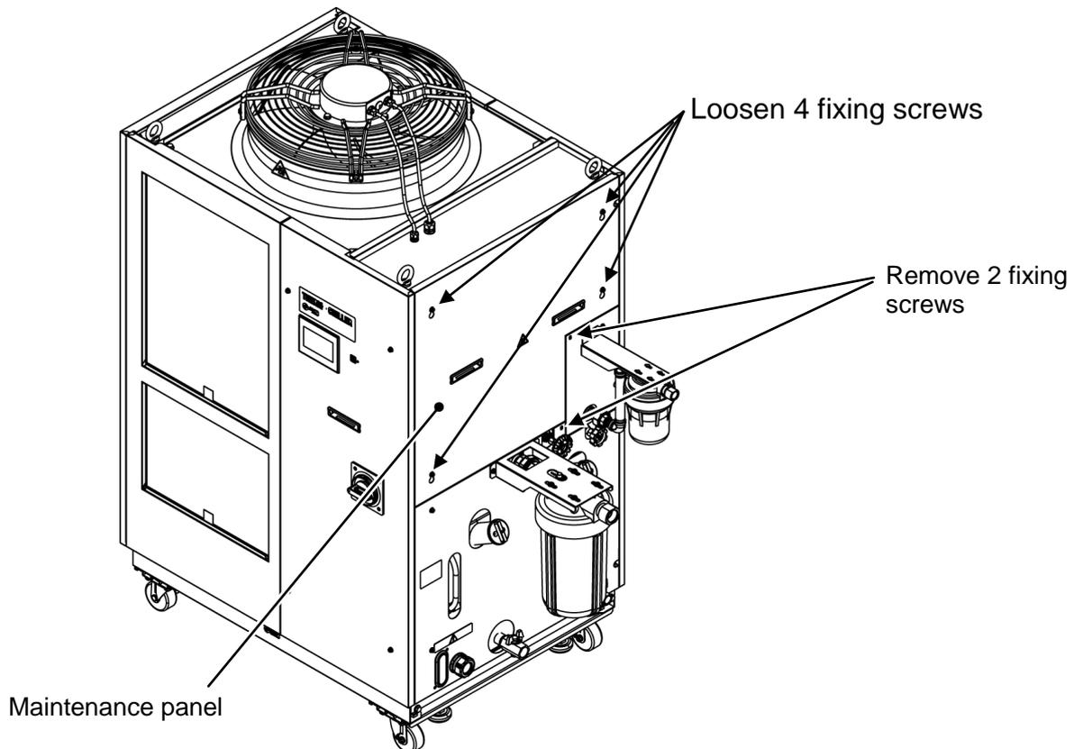
Fig. 7-5 Maintenance panel removal
