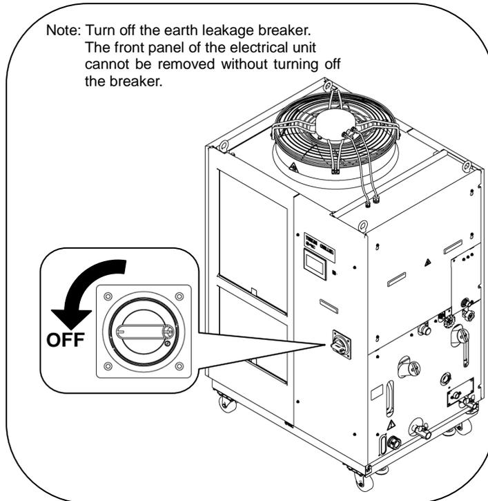
Fig. 3-6 Remove the front panel for the electrical unit
