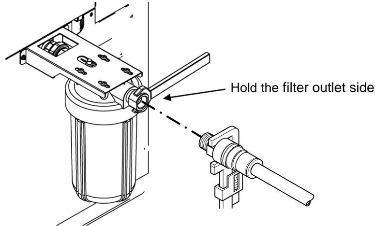
Fig. 3-17 Hold the filter outlet side
