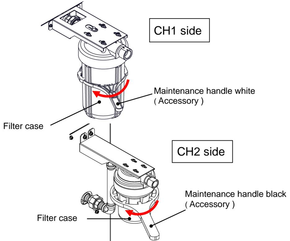
Fig. 7-3 Particle filter removal
