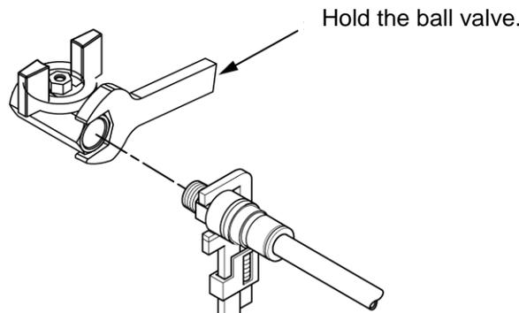
Fig. 3-18 Connection to the drain port
