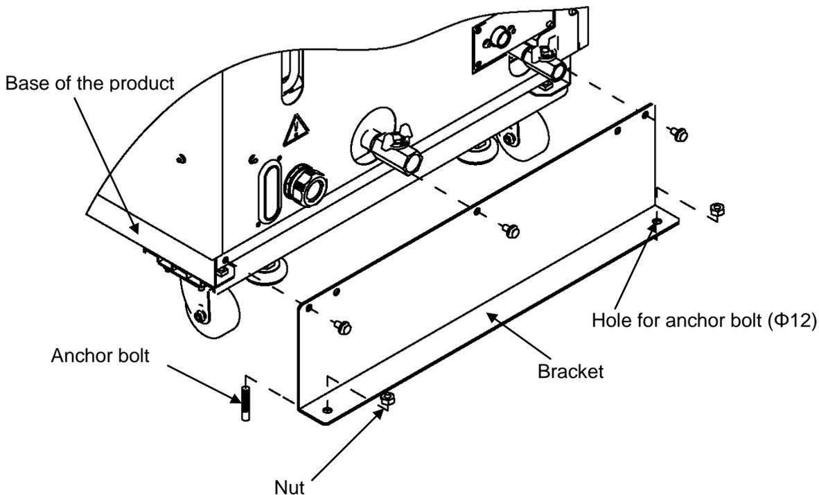
Fig. 3-4 Installation procedures
