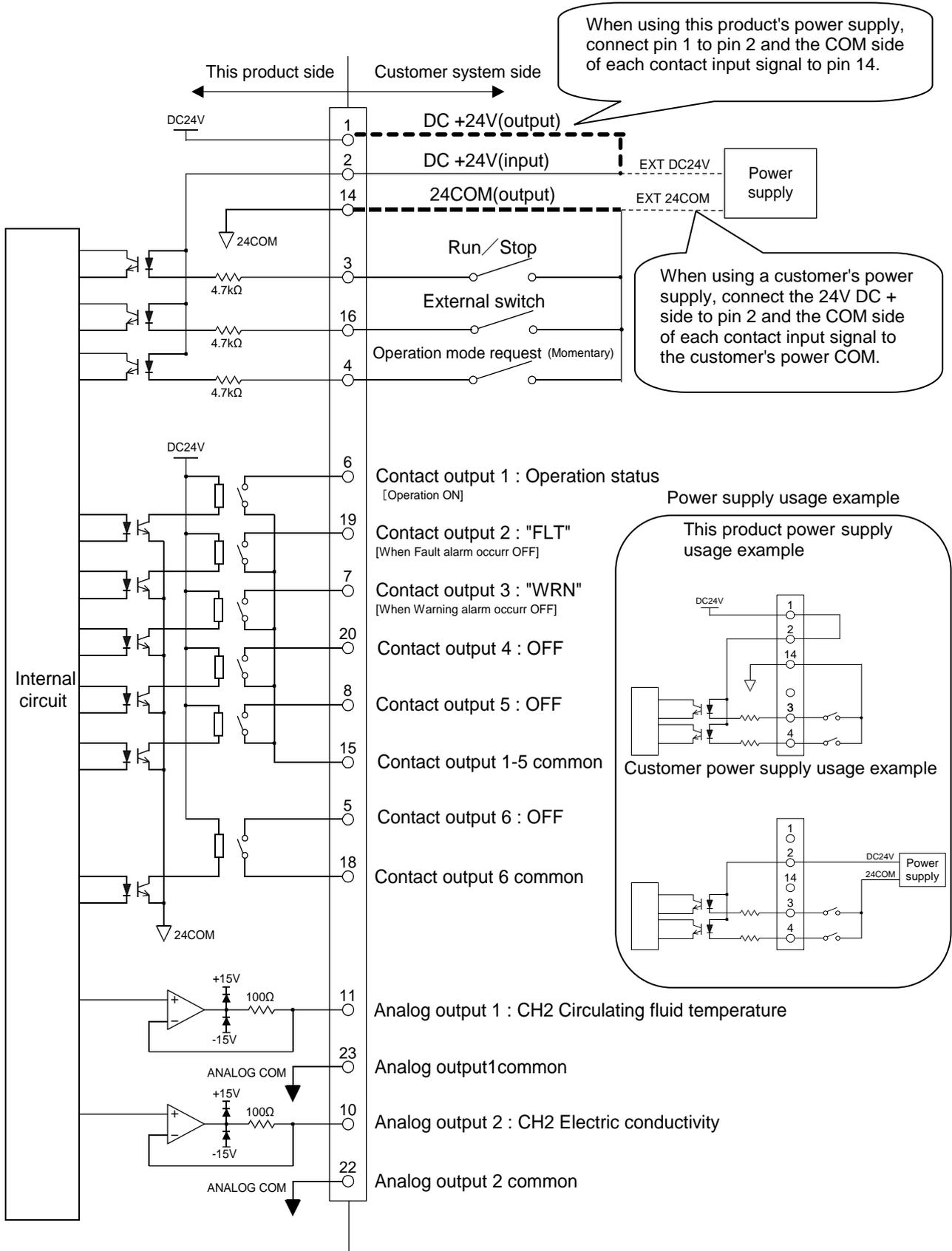
Fig. 3-10 Circuit diagram
