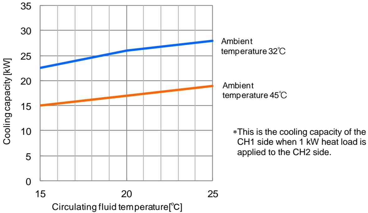
Fig. 8-7 Cooling Capacity (HRL300-A\*-20)
