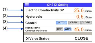
Electric conductivity and alarm (AL27) setting
